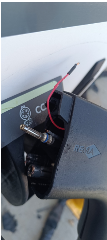
Exhibit E - Station 2607. Close view of physically open/damaged charging hardware with internal components visible.
