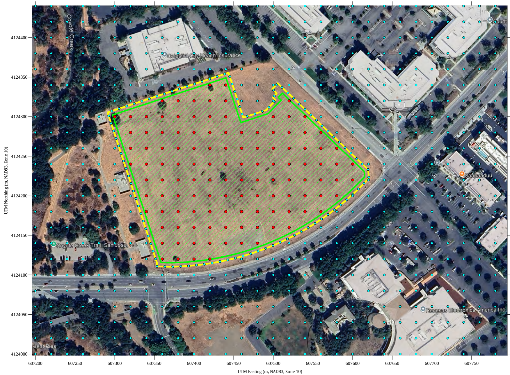
Figure AQ4-1 : Silver Creek Construction Modeling Red Points = Construction Stacks Cyan Points = Receptor Locations Green Hashed Area = Fugitive Area Source Yellow Line = Property Boundary
