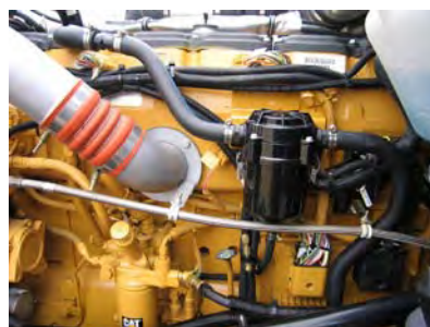
CCV4500 installed on a CAT engine.
