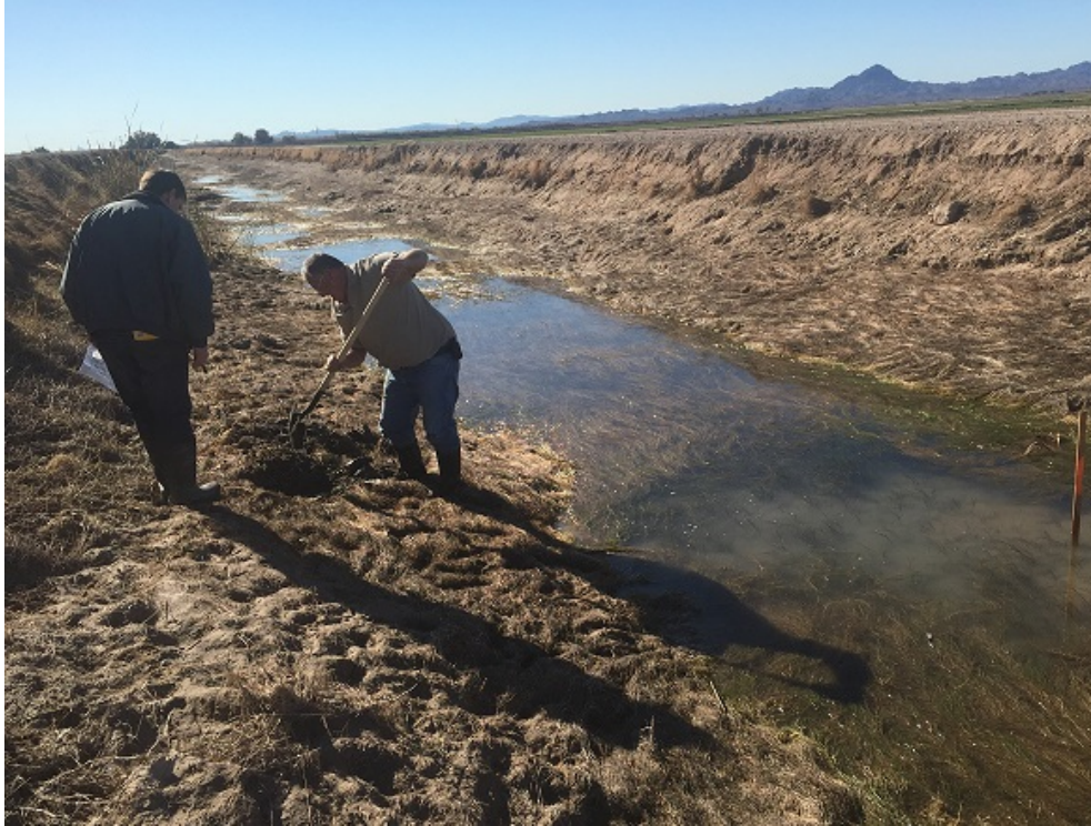
Figure 4. Samples Taken at Three Locations in the Side Slopes Because of Water in Canals
