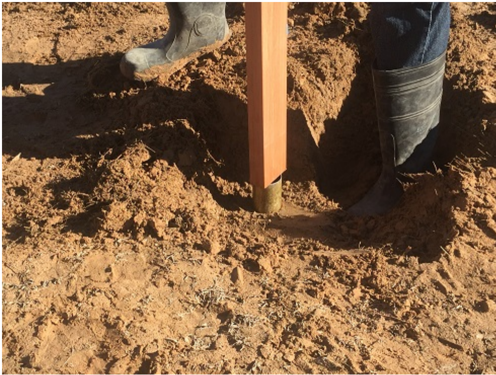
Figure 5. 2.5-inch-Diameter Brass Tube Inserted into Canal for Hydraulic Conductivity Sample
