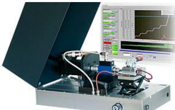
Electric Motor Test Bench
