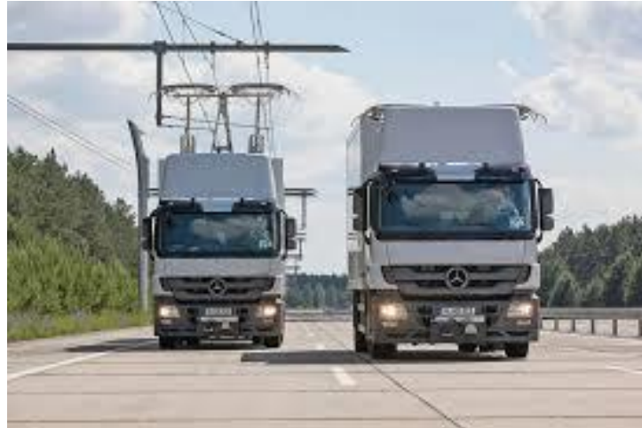
Figure 3.6 Siemens eHighways Concept (in prototype form, diesel-electric hybrid truck on the right)
