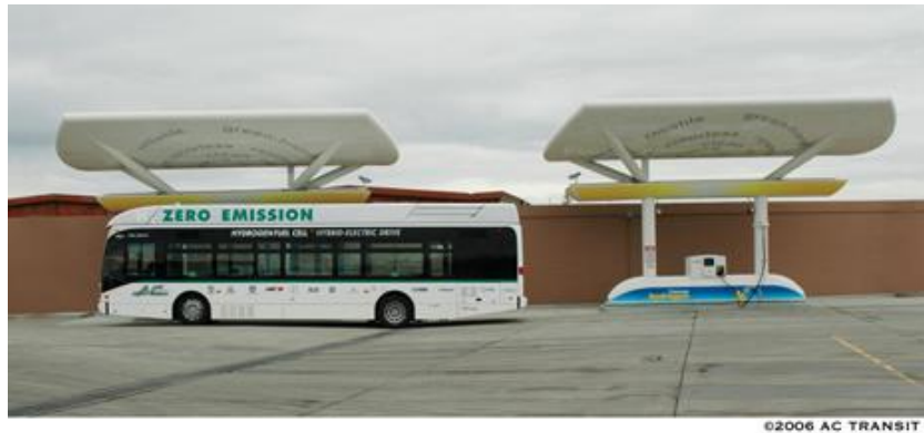
Figure 3.4 AC Transit Fuel Cell Bus at Chevron H2 Station, Oakland, CA
