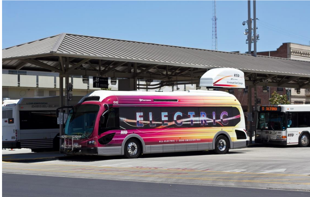
Figure 3.8 Proterra BEV Transit Bus Overhead Ultra-Fast Charger, Stockton, California
