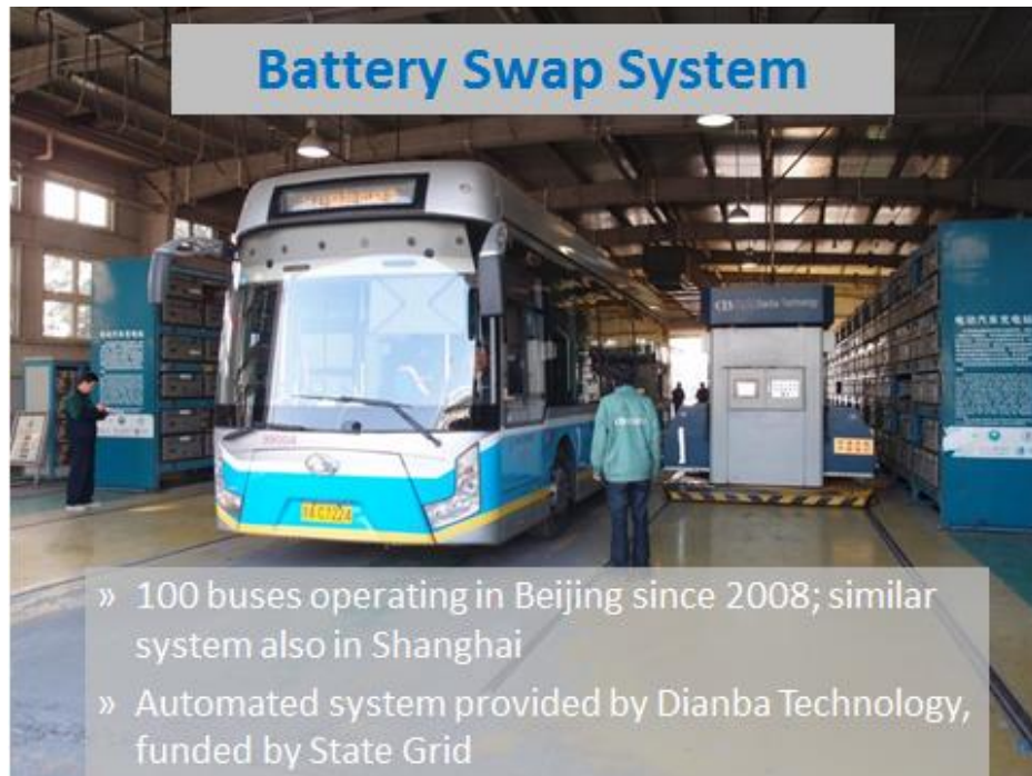
Figure 3.11 Battery Swap Systems, Automated System, China
