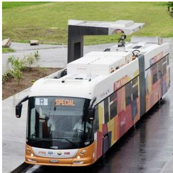
Figure 3.9 ABB “TOSA” Hybrid Transit Bus Overhead Ultra-Fast Charger, Geneva, Switzerland
