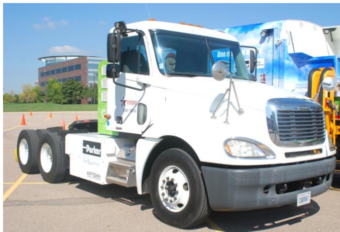
Figure 2.2 Turbine Range-Extender Electric Truck (Artisan/Capstone/Parker on a Freightliner Chassis)
