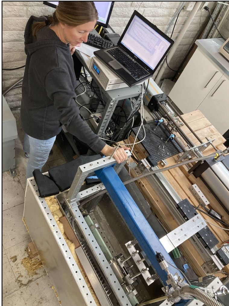
A staff member at General Engineering & Research works on the cryogenic magnetic refrigeration prototype.
