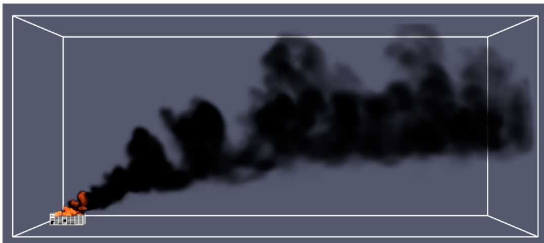
Figure 32. Plume development under a -10 K/km lapse rate.
