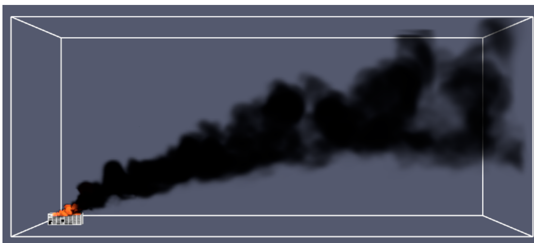
Figure 33. Plume development under a -20 K/km lapse rate.
