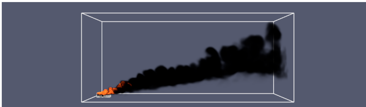
Figure 24. LFP flaming plume at 10 m/s, 22°C, and 2-hour duration.
