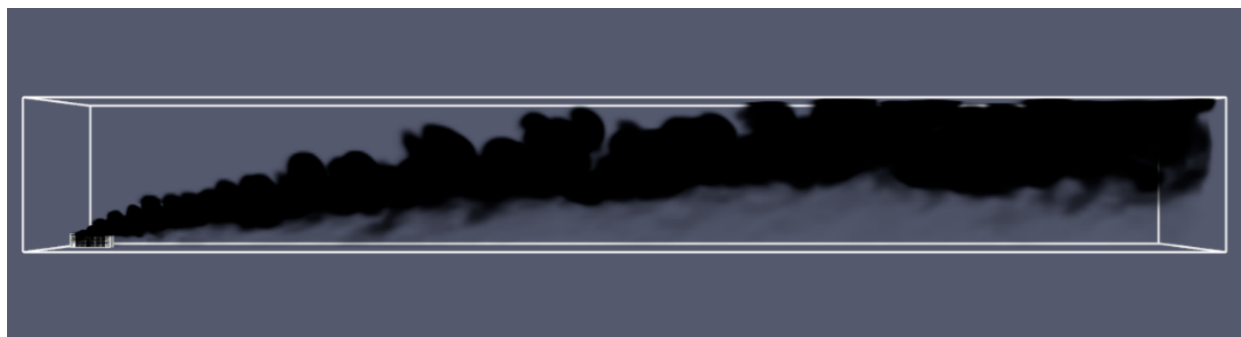
Figure 19. NMC non-flaming plume at 2 m/s, 22°C, and 0.5-hour duration.
