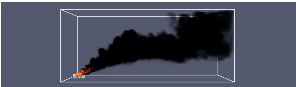
Figure 23. LFP flaming plume at 5 m/s, 22°C, and 2-hour duration.
