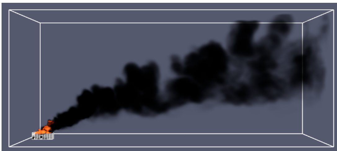
Figure 31. Plume development under a 12 K/km lapse rate.
