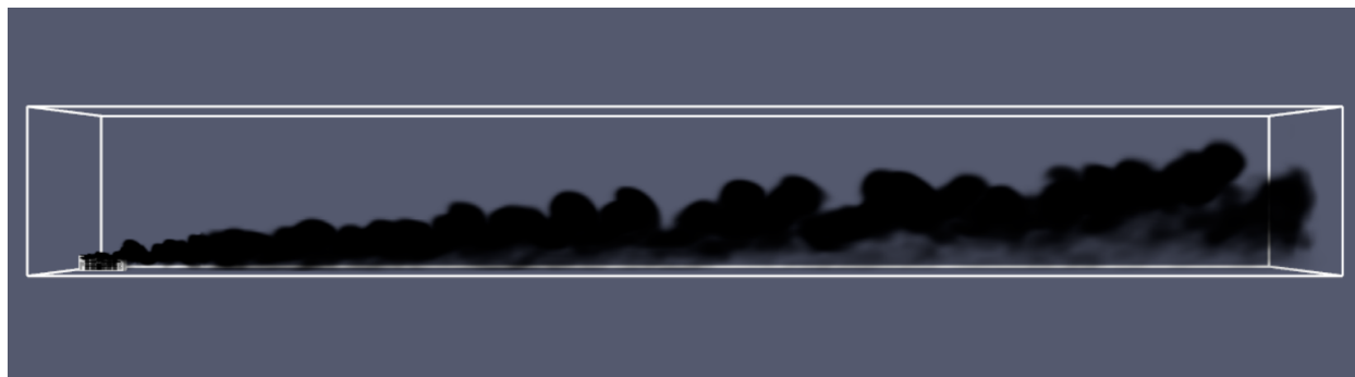
Figure 21. NMC non-flaming plume at 2 m/s, 22°C, and 2-hour duration.
