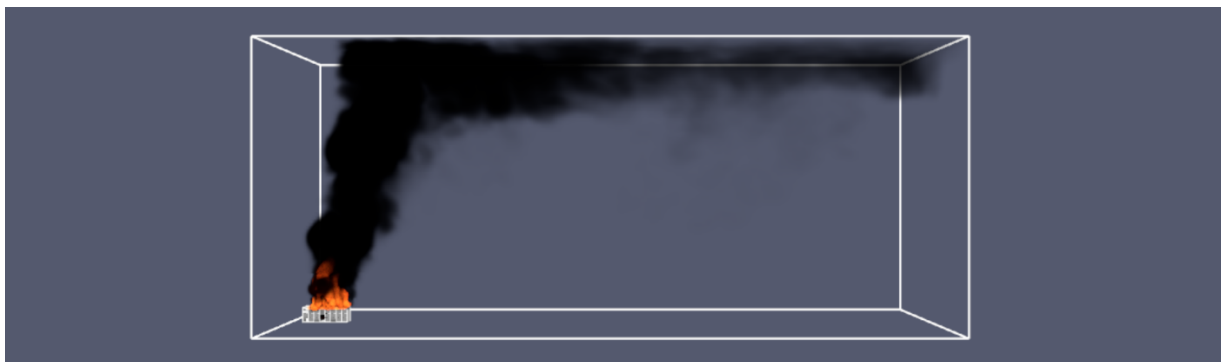
Figure 22. LFP flaming plume at 2 m/s, 22°C, and 2-hour duration.
