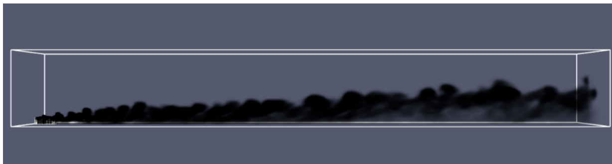
Figure 18. LFP non-flaming plume at 2 m/s, 22°C, and 6-hour duration.
