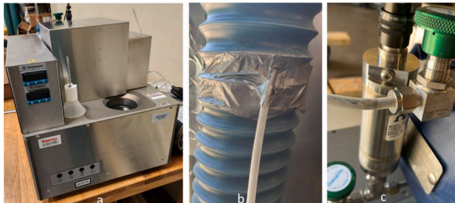
Fig. 2. Gas analysis setup with FTIR (a; Thermo Scientific Antaris IGS Analyzer, b; sample point from exhaust, c; FTIR gas inlet).
