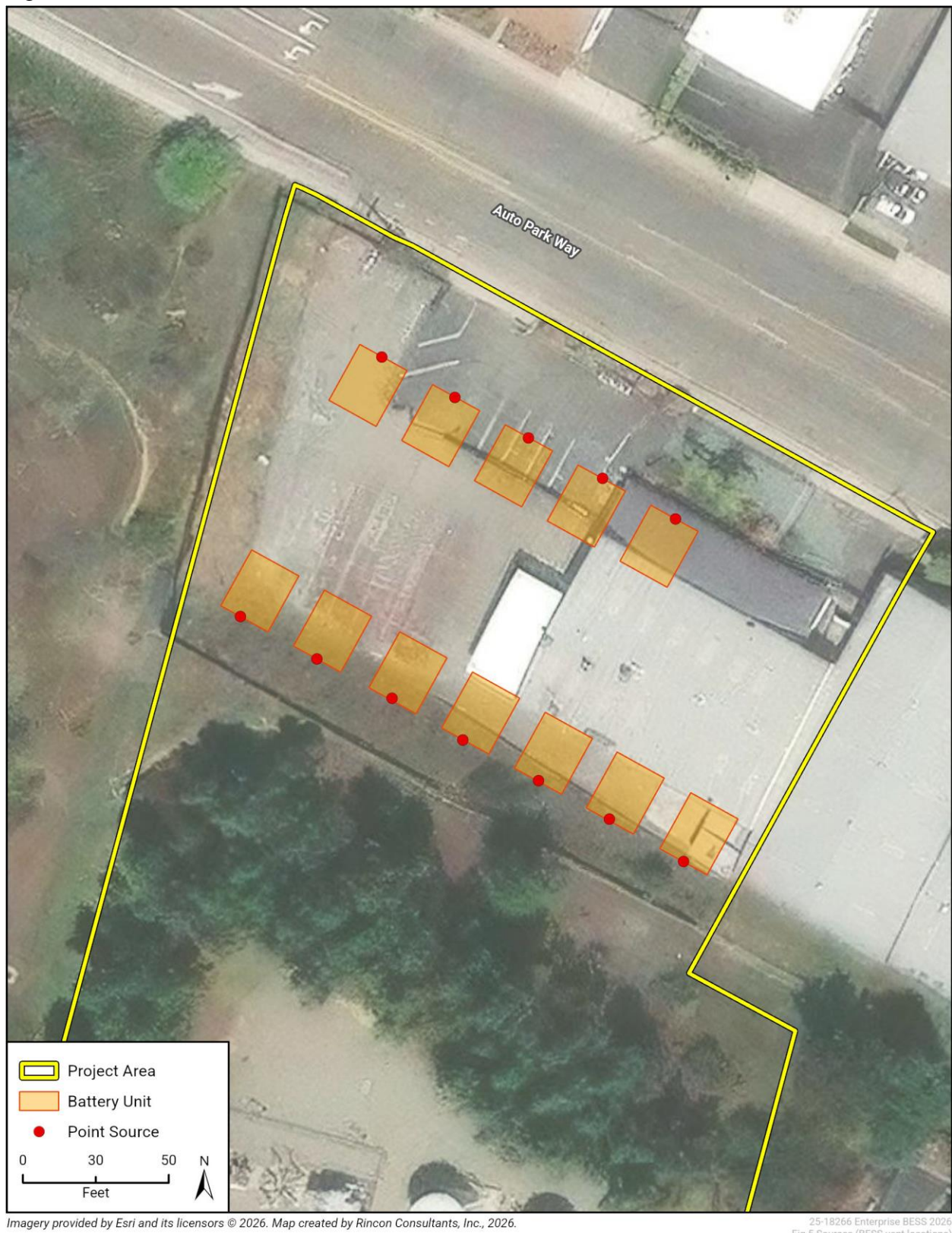
Figure 3 AERMOD Modeled BESS Vent Locations
