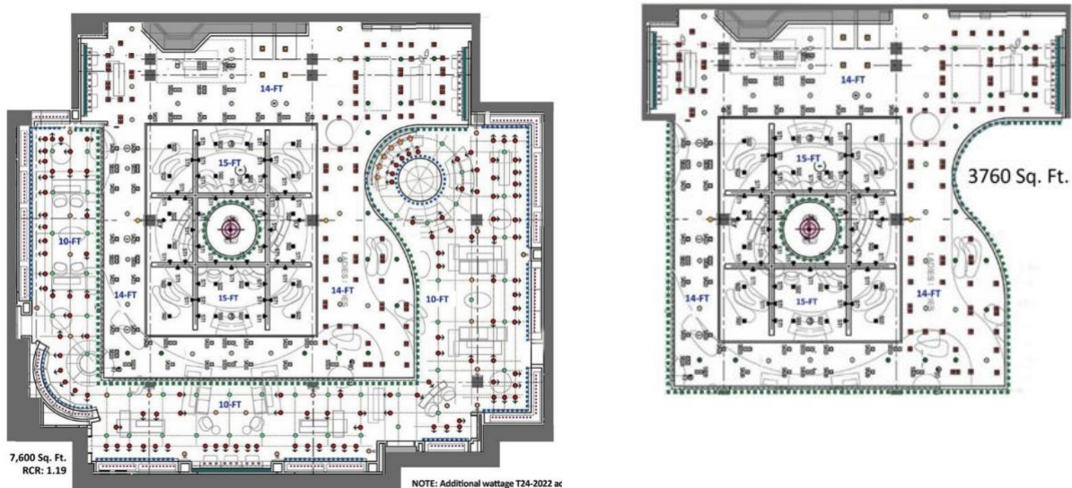
Figure 1: High-End Shoe Store And Example Of Problematic Partial Retrofit With Few Full Height Walls And Significant Areas Of Bulkhead Lighting
