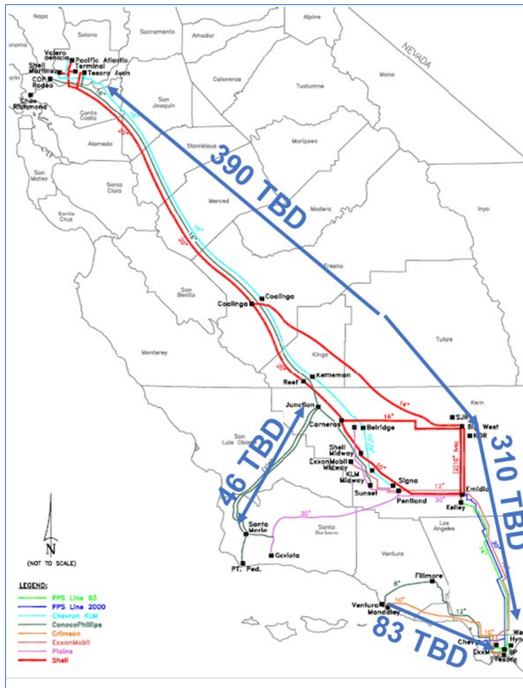
Figure 7 - Location, alignment and carrying capacity of key crude oil pipeline infrastructure
