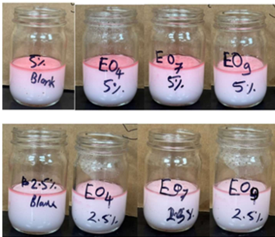
Figure 17. 5-Minute static emulsion stability screening test for 5% and 2.5% extractant concentration. Visual phase-separation comparison of non-ionic surfactants from left to right blank (water), SF-3, SF-4 and SF-5.
