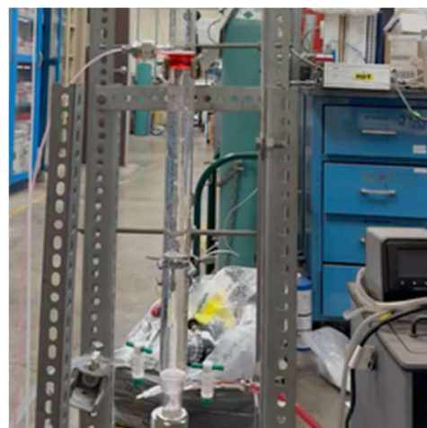
A ) Schematic of experimental setup B ) photograph of the extraction experiment Figure 11. A) Schematic of the semi-continuous bubble-contacting column for Zn extraction; B) photograph of the column during operation
