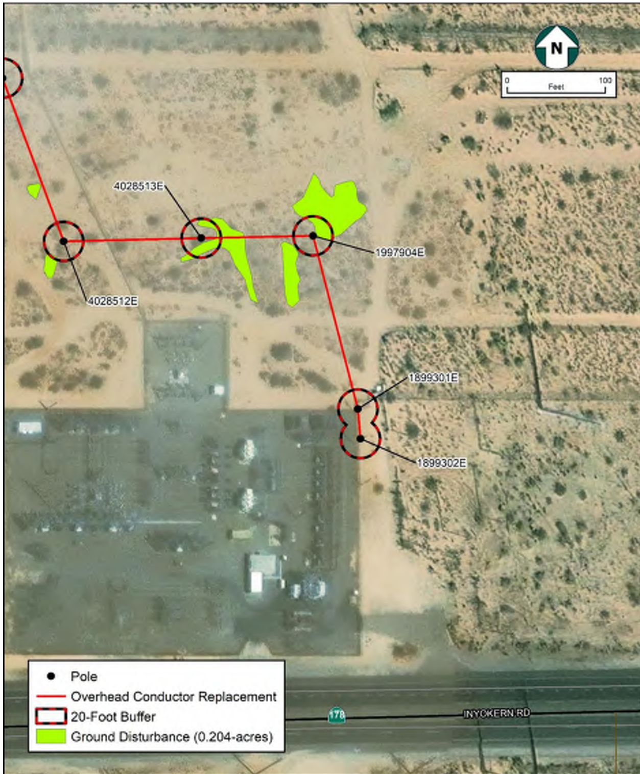
Figure 8 Habitat Disturbance SCE Pole Replacement and Upgrades in Support of RB Inyokern Solar Project, Kern County, California.
