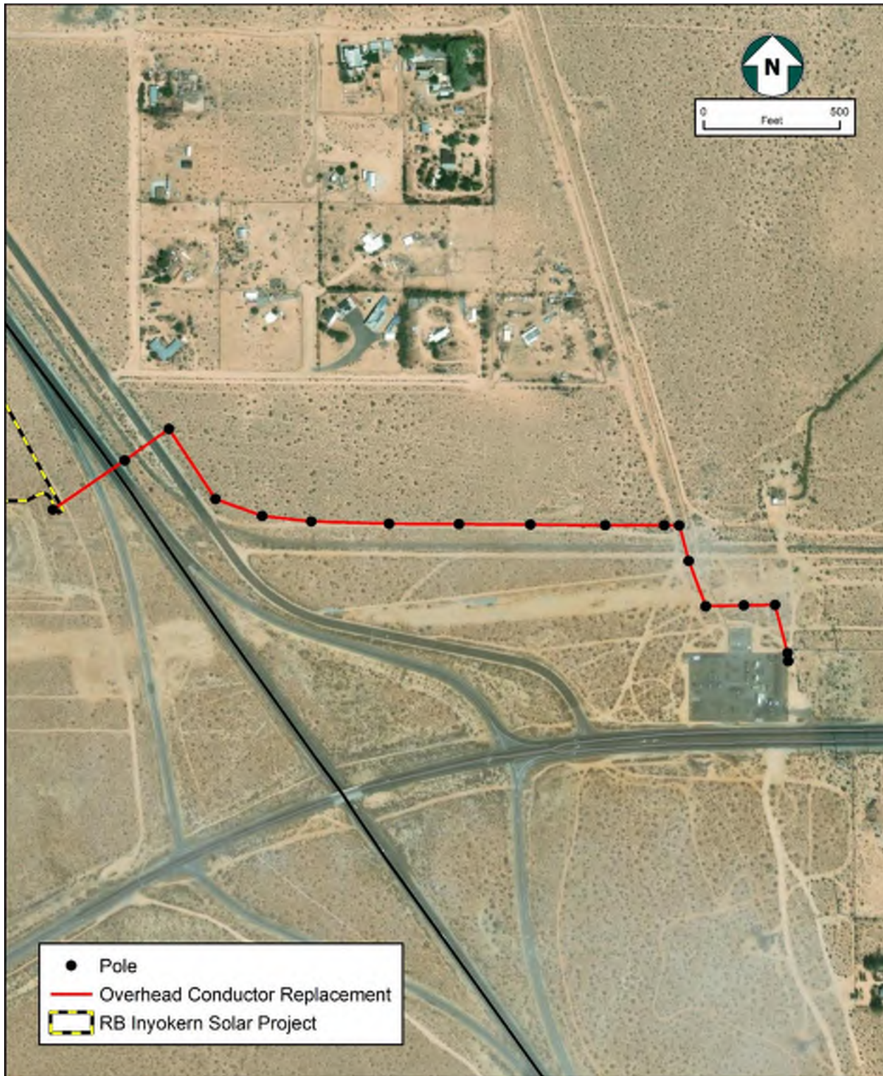
Figure 3 Project Site SCE Pole Replacement and Upgrades in Support of RB Inyokern Solar Project, Kern County, California.
