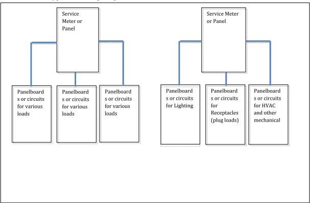
panel such that the load type can be studied independent of other loads. Note that either temporary metering or permanent metering can be used.
