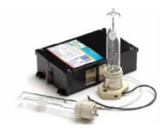
These systems have lamp/ballast **SYSTEM EFFICACIES** of **103-111 lm/watt** initial and 82-89 lm/watt at 12,000 hr ("mean") yet are only specified for dimming to 50-60% rated power. Considering that a lamp/ballast system operating at 82-89 mean lumens per watt and 60% power uses considerably less energy than a more typical metal halide system operating in the 54-68 mean (lamp ballast system) lumens per watt range which is allowed 50% power during dimming
