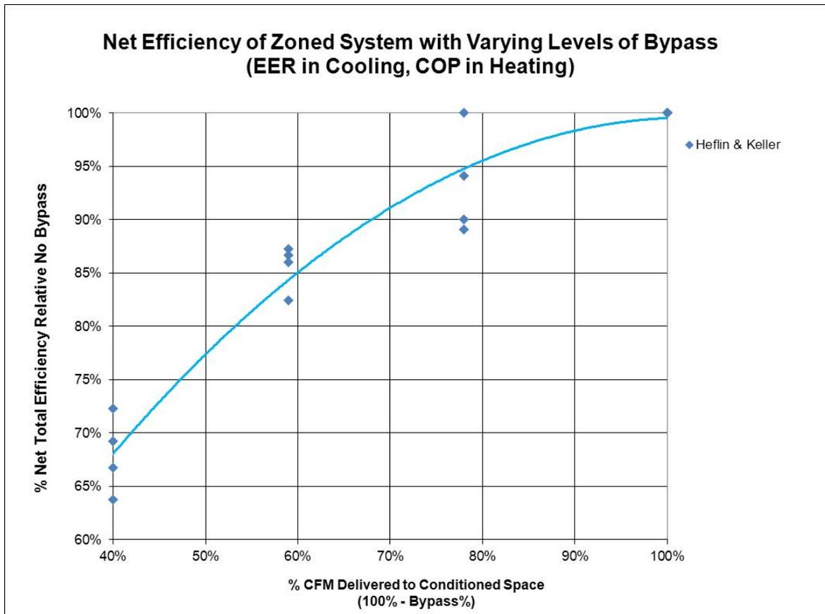
**Figure 2. Net Zoned System Efficiency with Bypass (Carrier Lab Data)**
