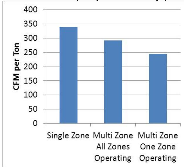
Figure 6. Airflow Reduction with Multi-Zoned HVAC Systems
