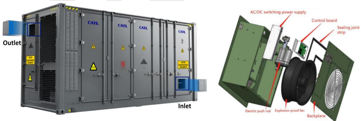
Figure 5. Explosion Control System Inlet/Outlets (Left) And Exhaust Fan (Right)
