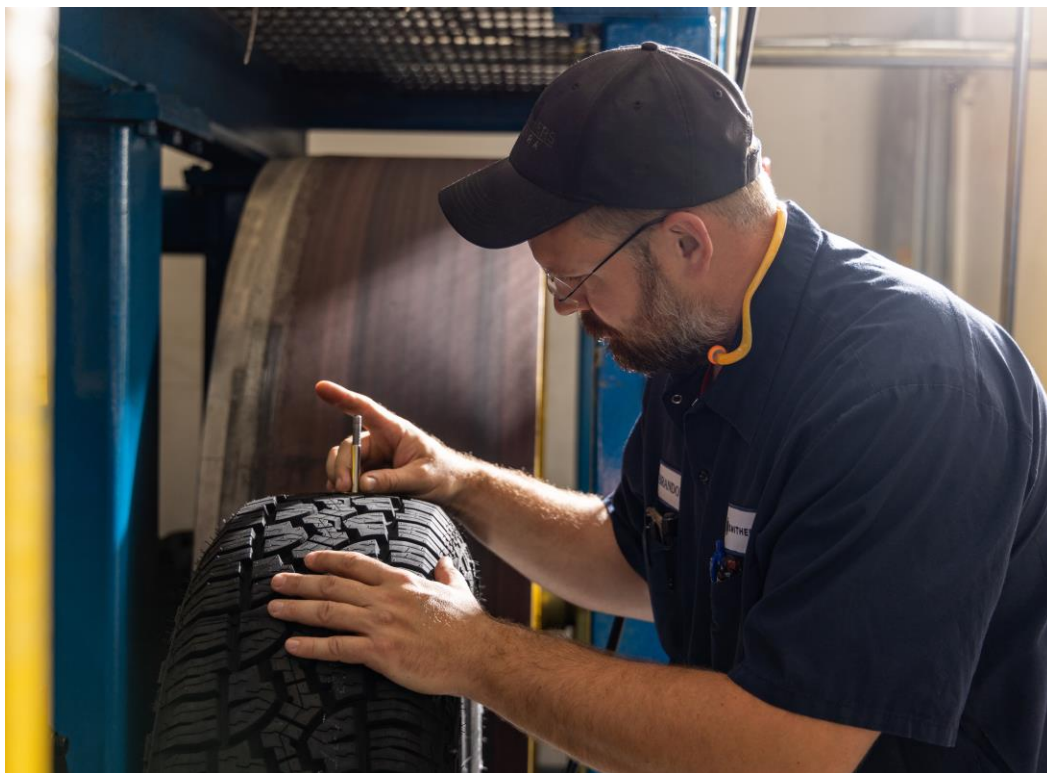
Photograph A5.4: Measuring Tread Depth
