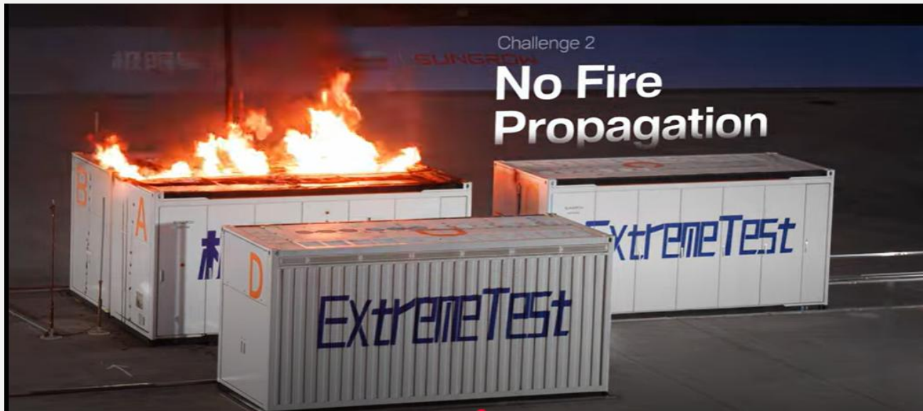
Exhibit 1. Sungrow Power Titan II Large-Scale Burn Test
