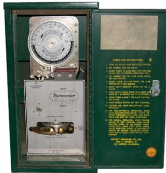
Figure 2-3: 1950s Landscape Irrigation Controller
