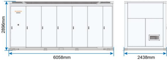
Figure 2-3 Dimensions of battery container
