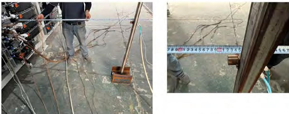
**Figure C11.** Heat Flux gauges in the center of the accessible mean of egress (distance from initiating unit: 1,520 mm)
