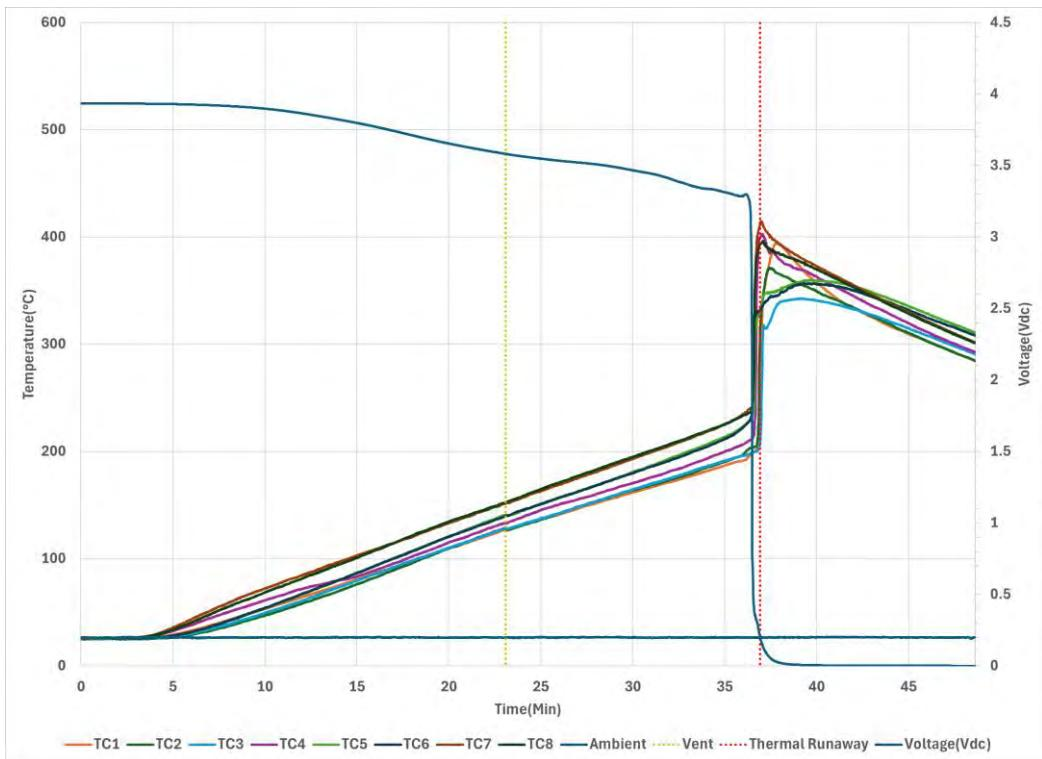
Figure C1: Sample 1 – Thermal Runaway &amp; Vent Temperature
