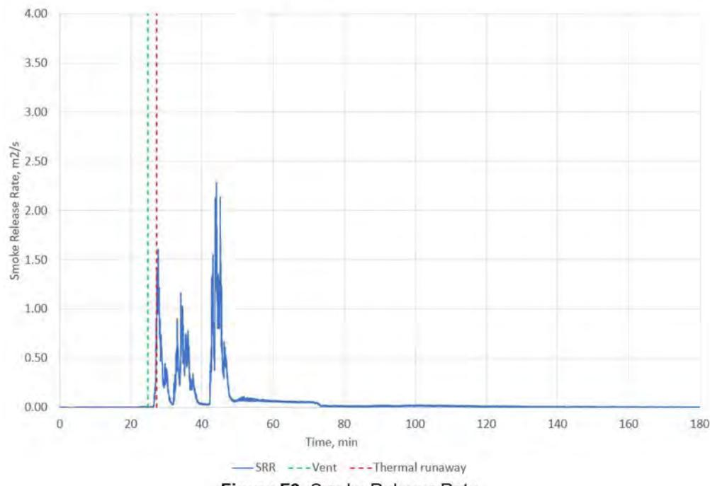
**Figure F3. Smoke Release Rate**
