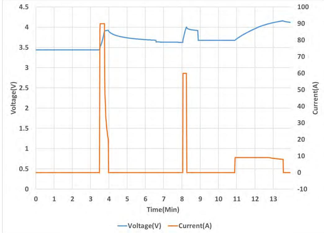
Figure A6: Sample 1- Charging and Topp-off Profile
