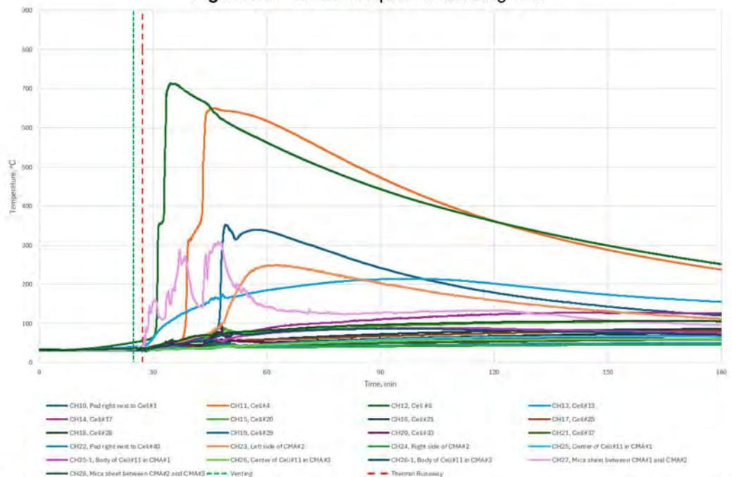
**Figure D2.** Channel of Thermocouples internal of Module excluding the initiating Cell (Cell#11)
