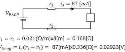
Figure 3. Voltage Drop Calculation
