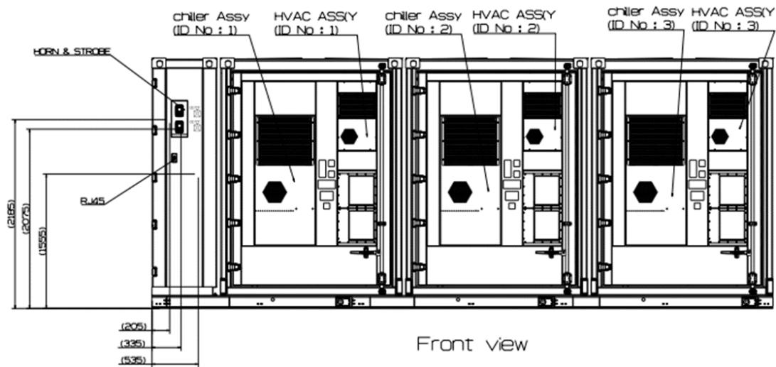
Figure 17. Front View of JF2 DC/AC LINK
