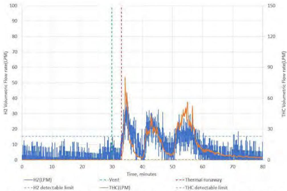
**Figure F1.** Volumetric flow rates of gases over the duration of the unit test (H<sub>2</sub> and THC)
