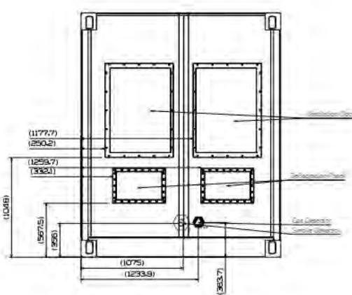
Figure 20. Location of Smoke Detector and Gas Detector (M-LINK, Top view)
