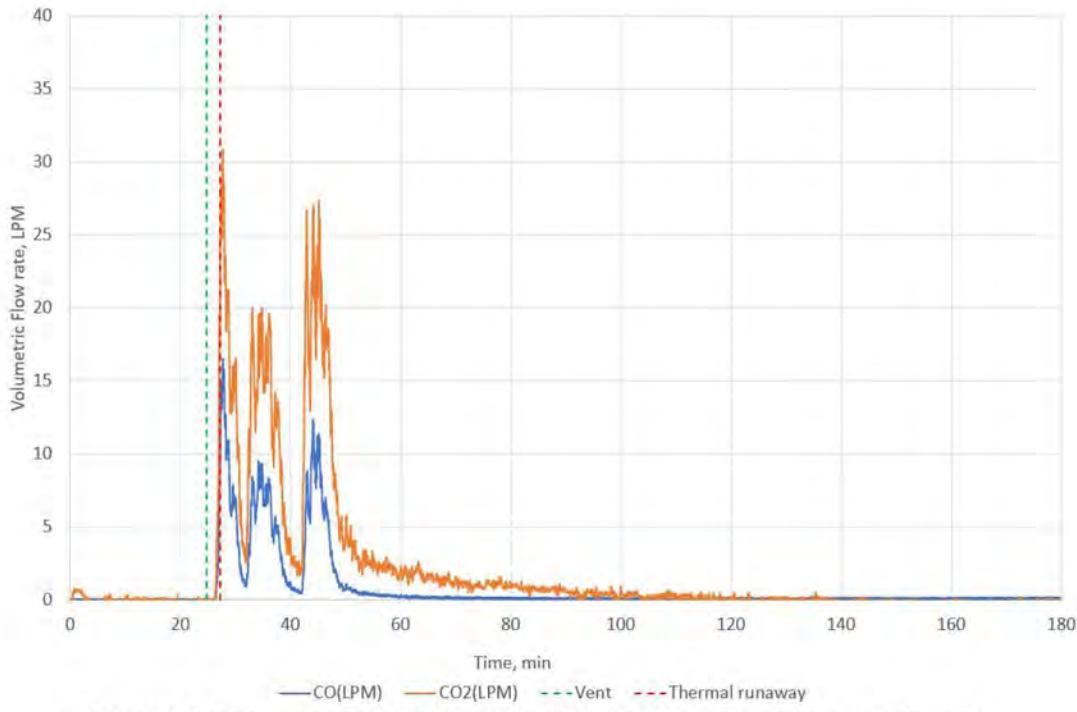
**Figure F2. Volumetric flow rate of gases (Carbon Monoxide and Carbon Dioxide)**
