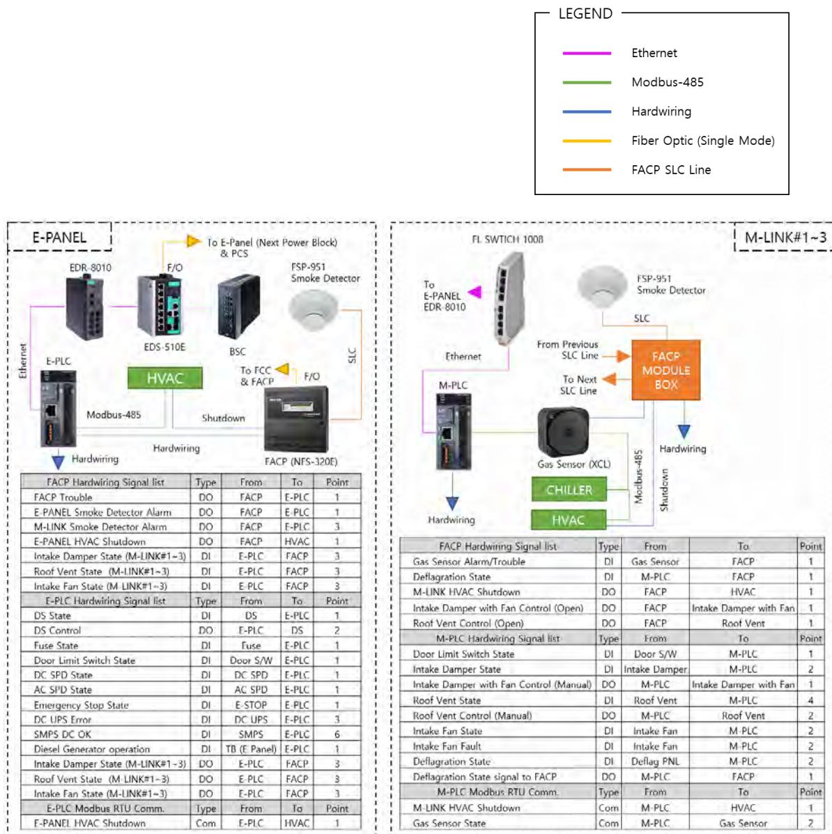
Figure 15. JF2 DC/AC LINK 5.1 Fire Safety Architecture (Communication)
