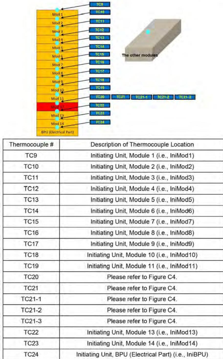
Figure C5. <sup>5</sup>Thermocouple Locations for the Initiating Unit
