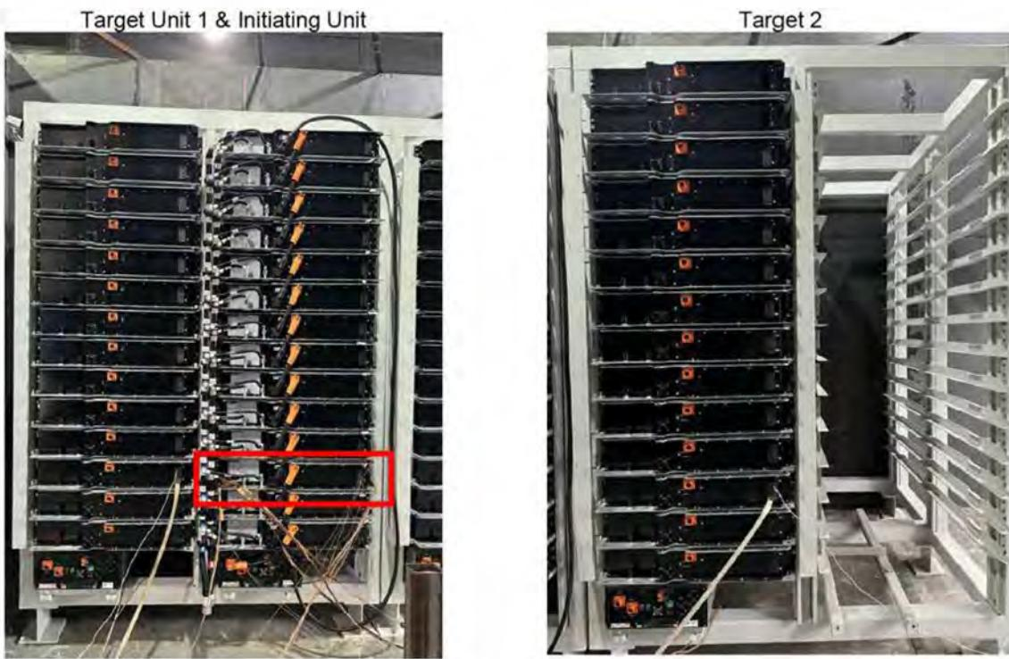
**Figure B1.** Photos of the Initiating and Target Units<sup>3</sup> / Initiating module (Third module from the bottom)
