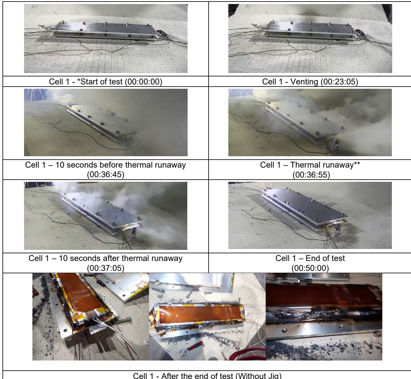
\*Note: Plate fixture is the jig for preventing swelling of cell to simulate the constraint in BESS Modules.
