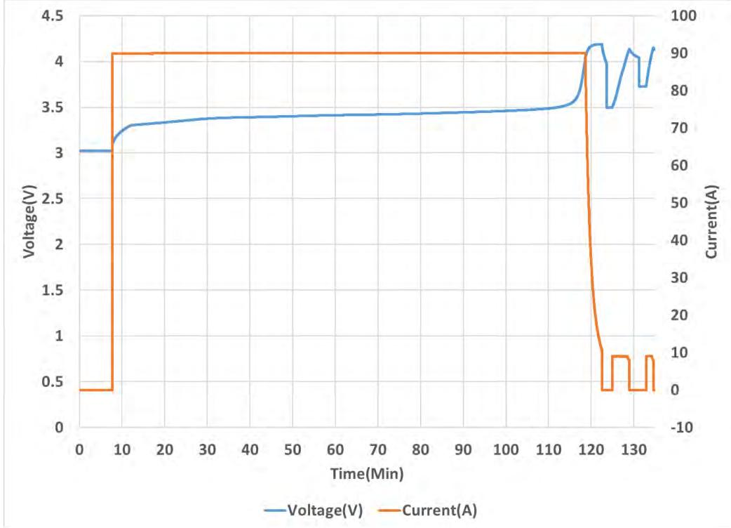
Figure A8: Sample 3- Charging and Topp-off Profile
