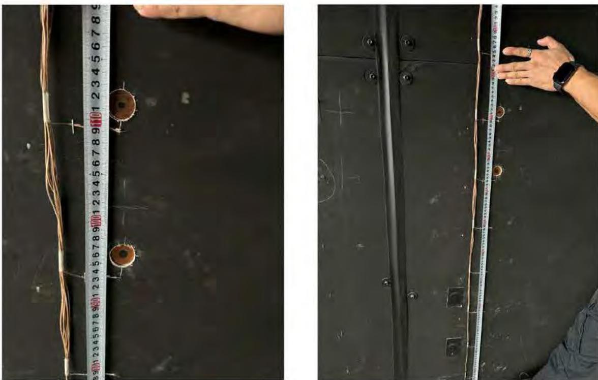
Figure C10. Heat Flux installed on the front wall
