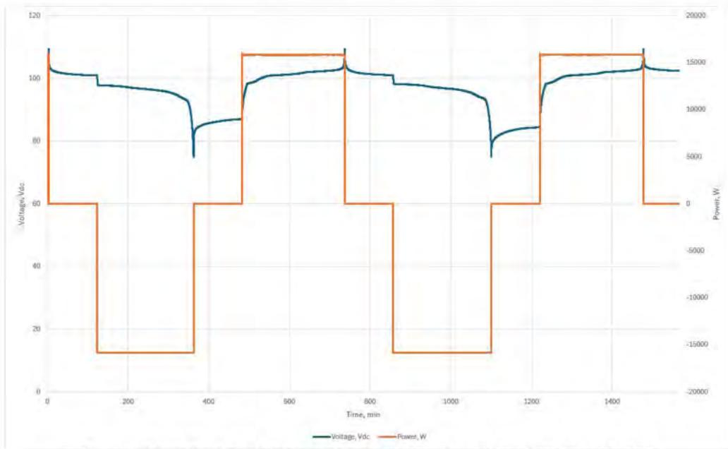
**Figure A1. 2 Cycles of Charging and Discharging on the initiating Module**
