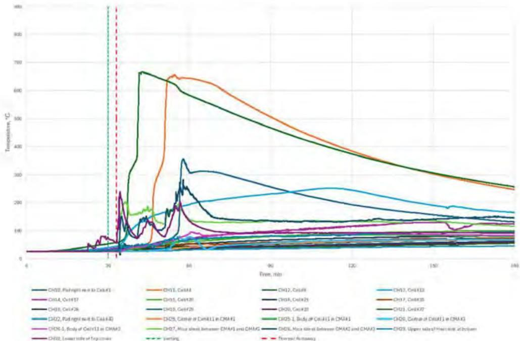
**Figure D2. Thermocouples inside of the initiating module**
