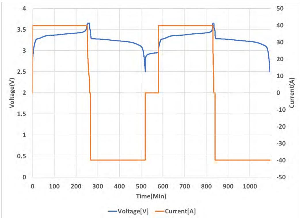
Figure A2: Sample 2 - Cell Conditioning Profile
