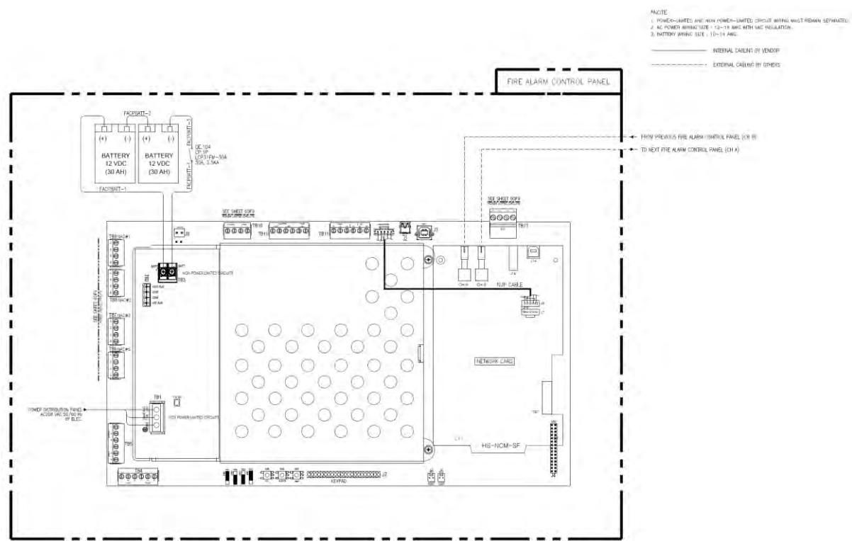
Figure 9. FACP Connection Diagram
