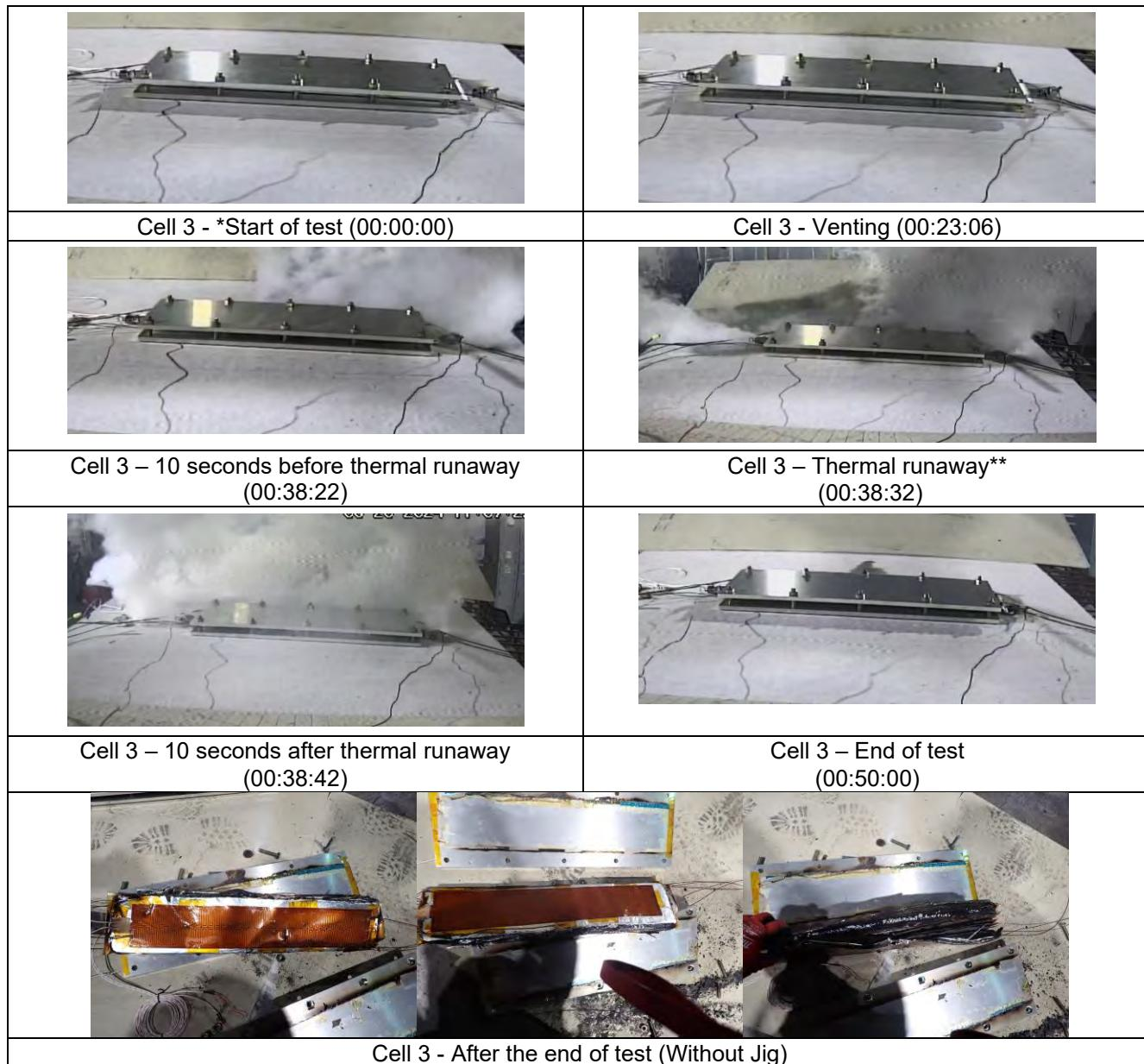
\*Note: Plate fixture is the jig for preventing swelling of cell to simulate the constraint in BESS Modules.
