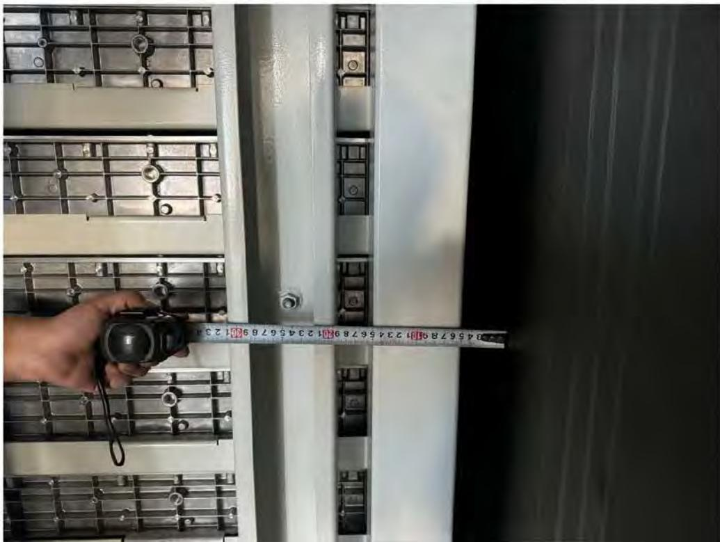
**Figure C13.** Distance from Rear Wall to Rear of Units. (distance from initiating unit: 500 mm)
