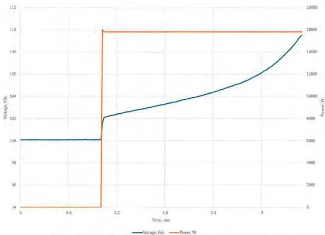
Figure A27. Module 14 (i.e., Mod 14) Charge Top-off on the test date
