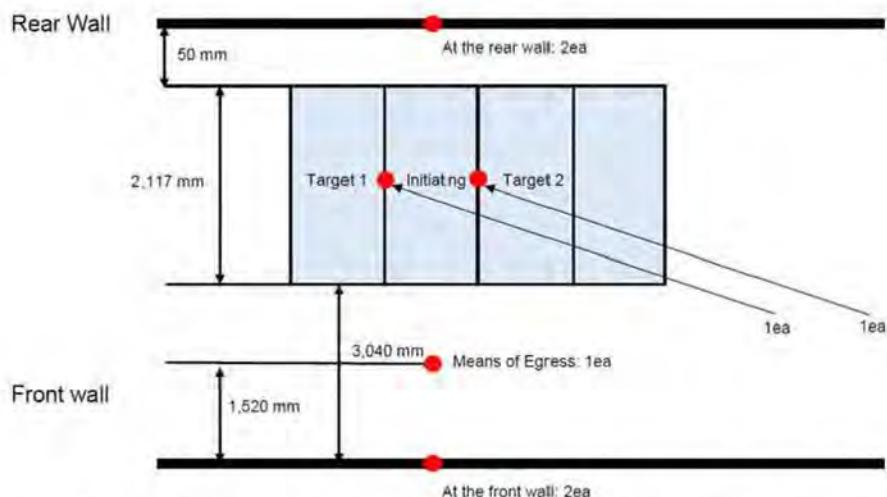
**Figure C1. Overall test installation layout & Heat Flux Gauge Plan**
