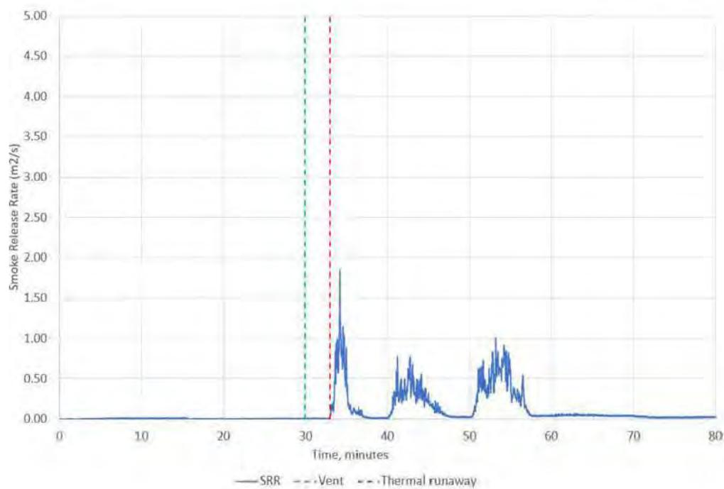
**Figure F3. Smoke Release Rate**
