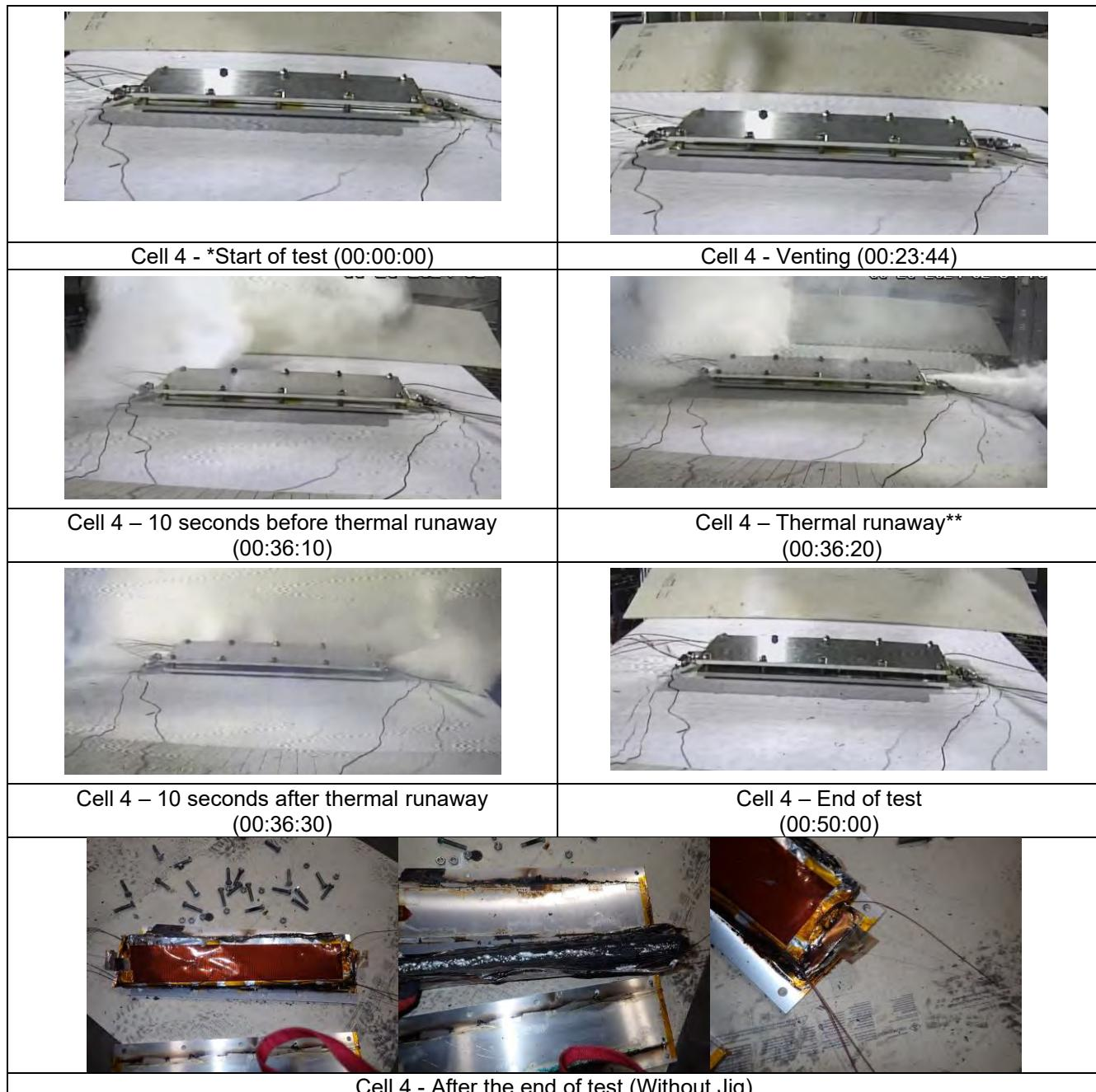
\*Note: Plate fixture is the jig for preventing swelling of cell to simulate the constraint in BESS Modules.
