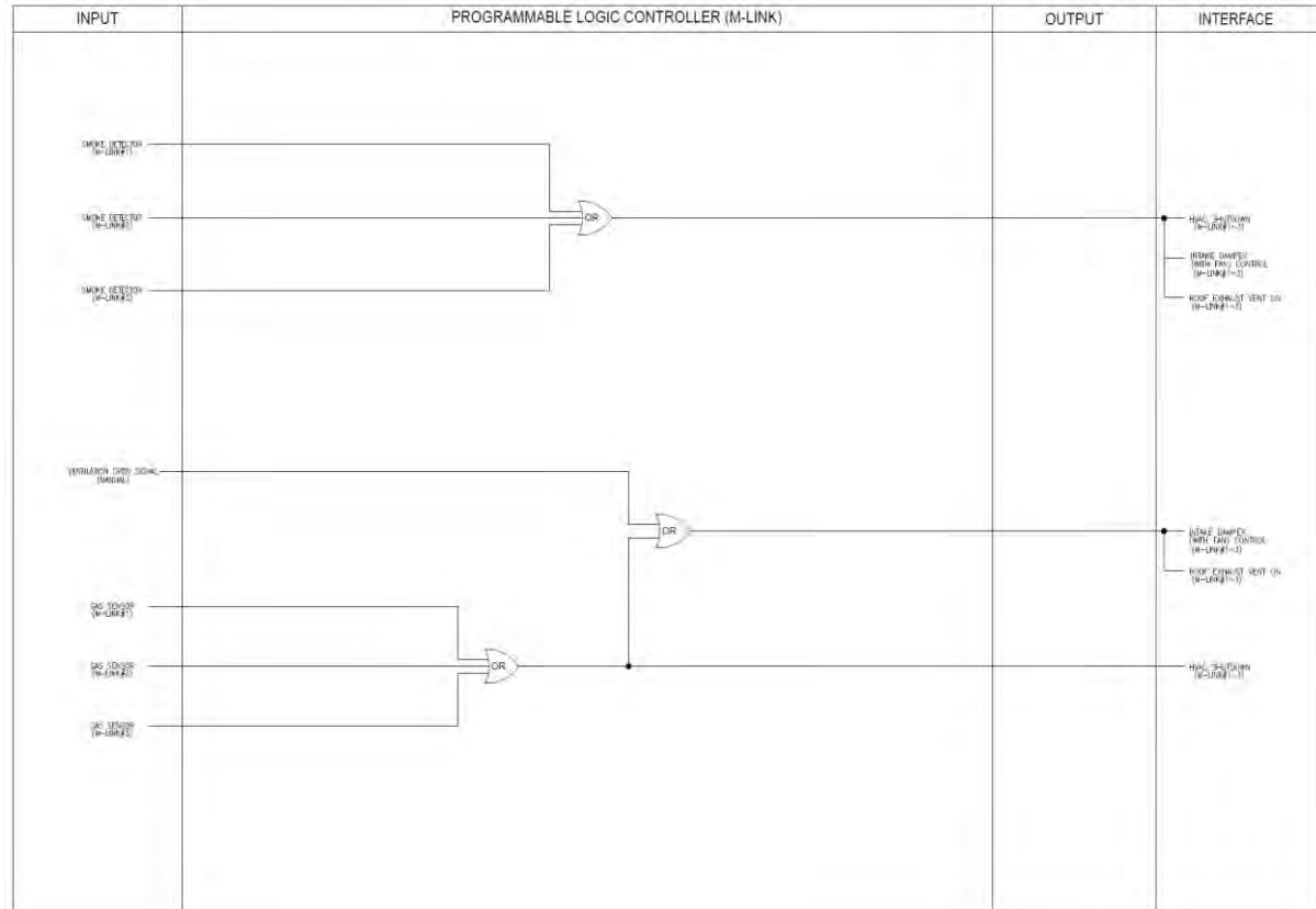
Figure 6. Fire Safety Logic of PLC (M-LINK)
