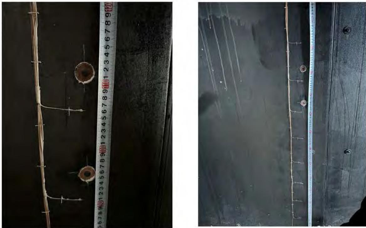
Figure C9. Heat Flux installed on the rear wall
