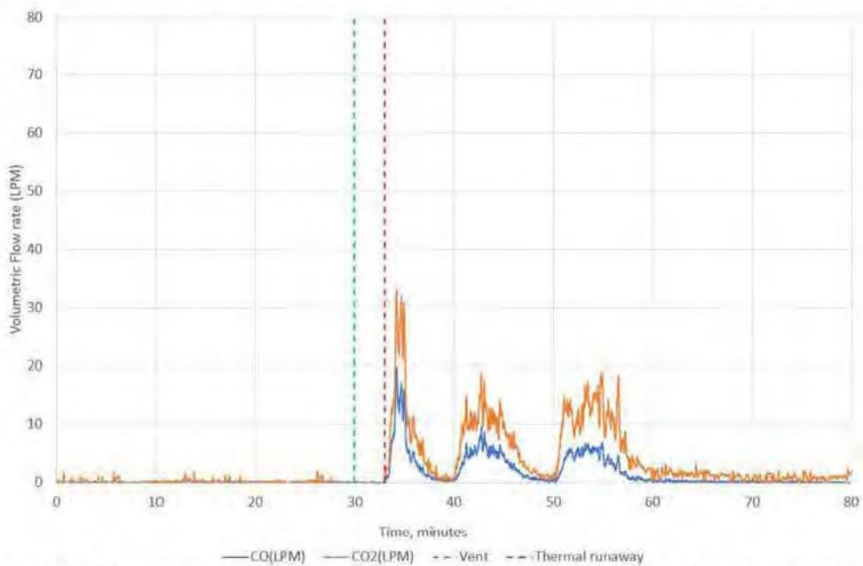
**Figure F2.** Volumetric flow rates of gases over the duration of the unit test (CO and CO<sub>2</sub>)
