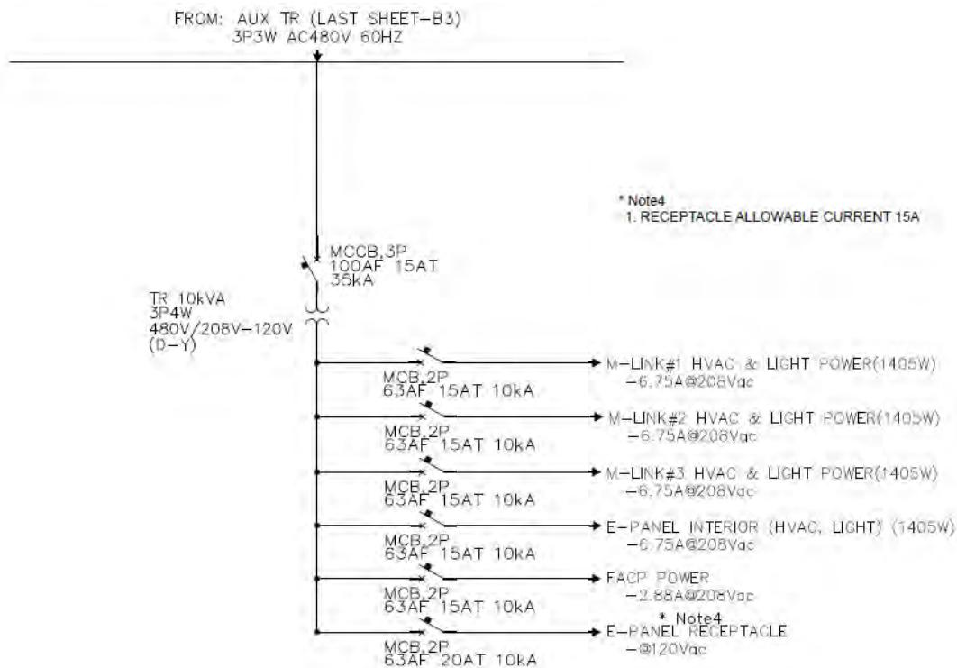
Figure 10. SLD (Breaker for FACP power)
