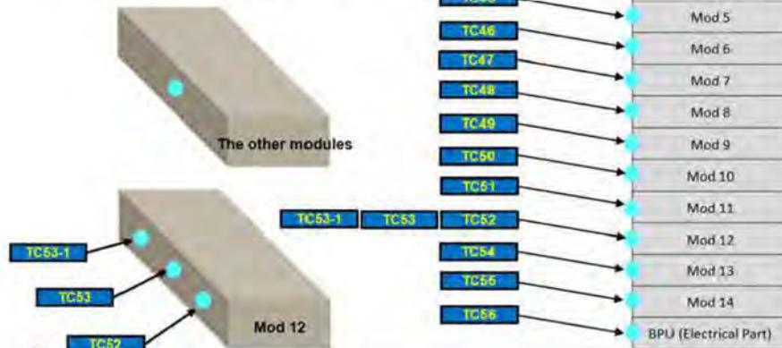
Figure C7. Thermocouple Locations for the Target Unit 2
