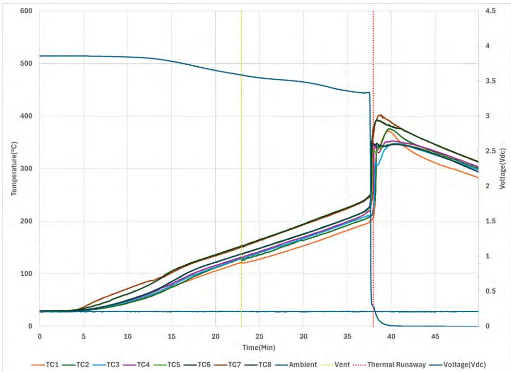
Figure C2: Sample 2 – Thermal Runaway &amp; Vent Temperature
