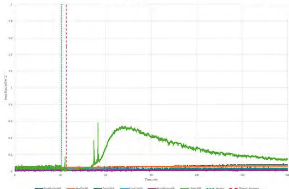
Figure D8. Heat Flux Measurements during the Unit Test (Targets and Walls)
