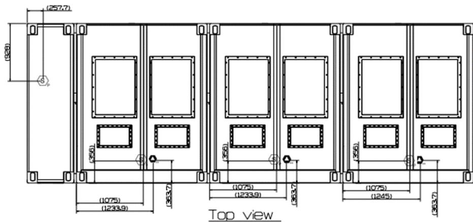
Figure 18. Top View of JF2 DC/AC LINK
