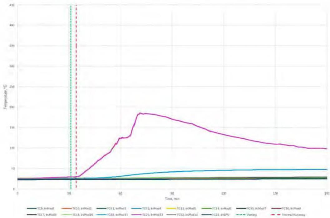
Figure D4. <sup>6</sup>Thermocouples on Modules in Initiating Unit
