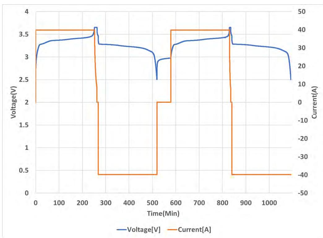
Figure A5: Sample 5 - Cell Conditioning Profile
