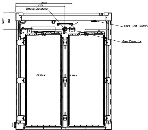
Figure 21. Location of Smoke Detector and Gas Detector (M-LINK, Front view)
