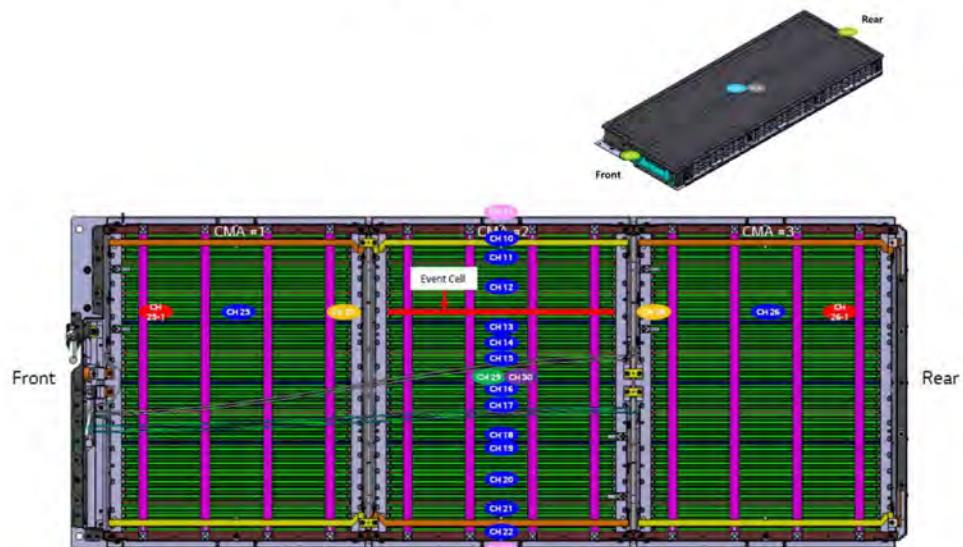
Figure C2. <sup>2</sup>Module cell and components instrumentation
