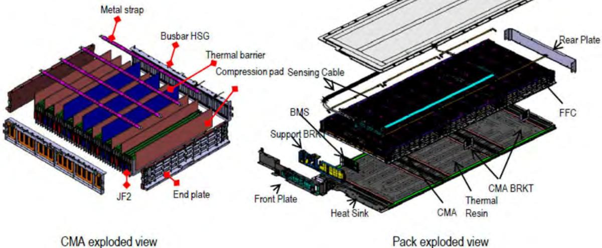
Figure B2. Exploded view of <sup>1</sup>Module and CMA
