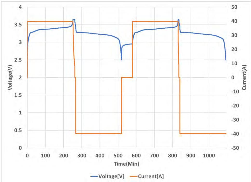
Figure A1: Sample 1 - Cell Conditioning Profile
