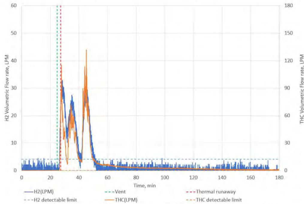
**Figure F1. Volumetric flow rate of gases (Total Hydrocarbon and Hydrogen)**
