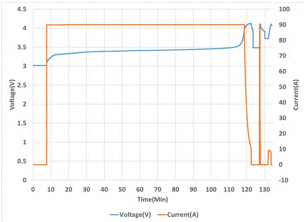
Figure A7: Sample 2- Charging and Topp-off Profile
