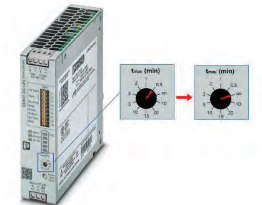
Figure 9: UPS Buffer Time Setting Adjustment
