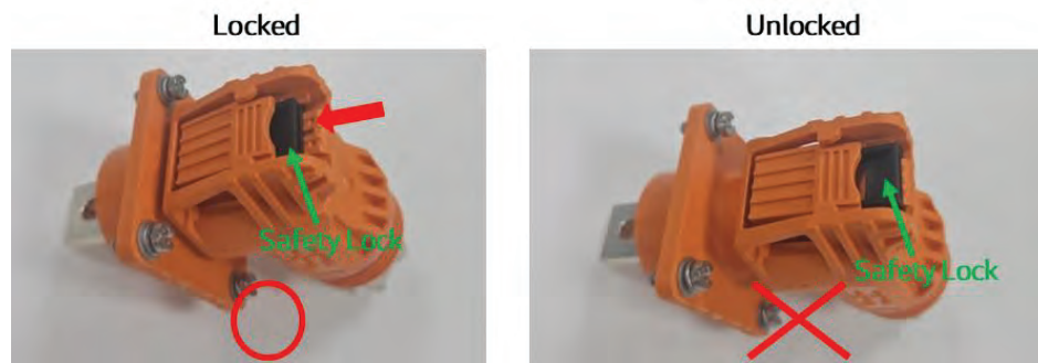
Figure 41: Pack to Pack cable connections
