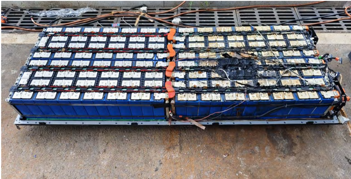
Figure 29. Photo 2 of initiating module after test
