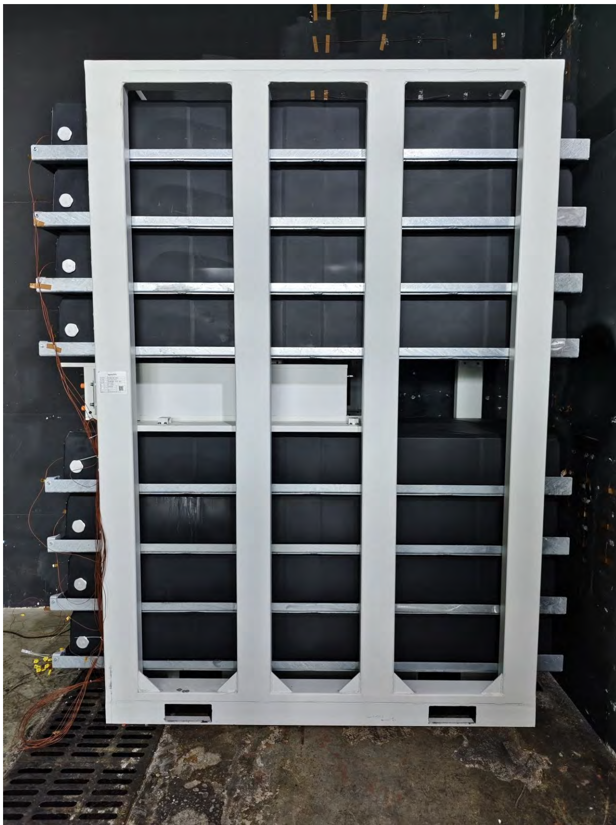
Figure 27. Photo 2 of initiating BESS Unit after test
