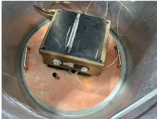
Figure 22: Sample 5 instrumented and inside gas test chamber
