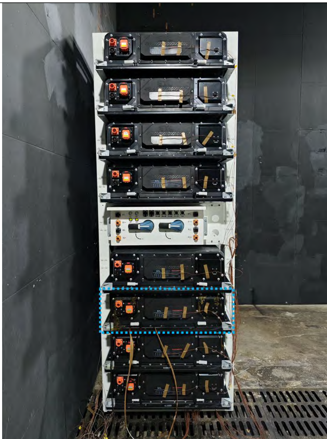
Figure 21. View of location of module that exhibited thermal runaway within the initiating unit
