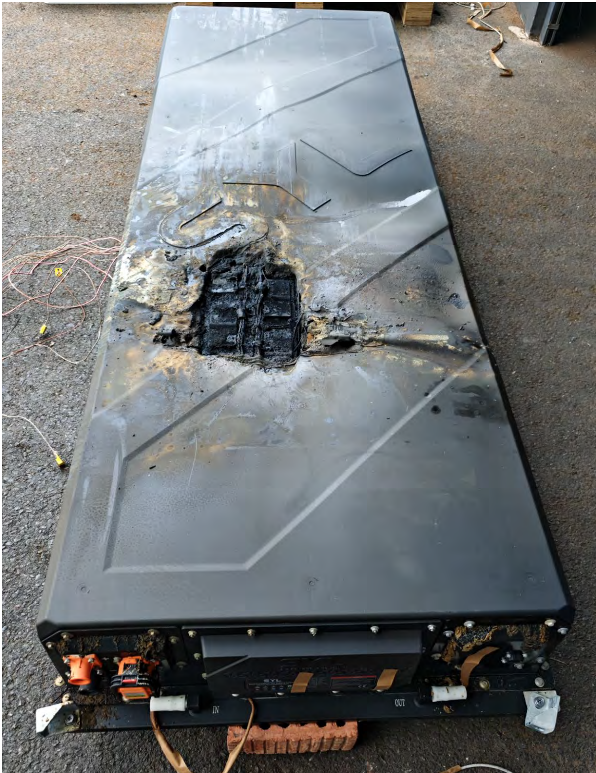
Figure 28. Photo 1 of initiating module after test
