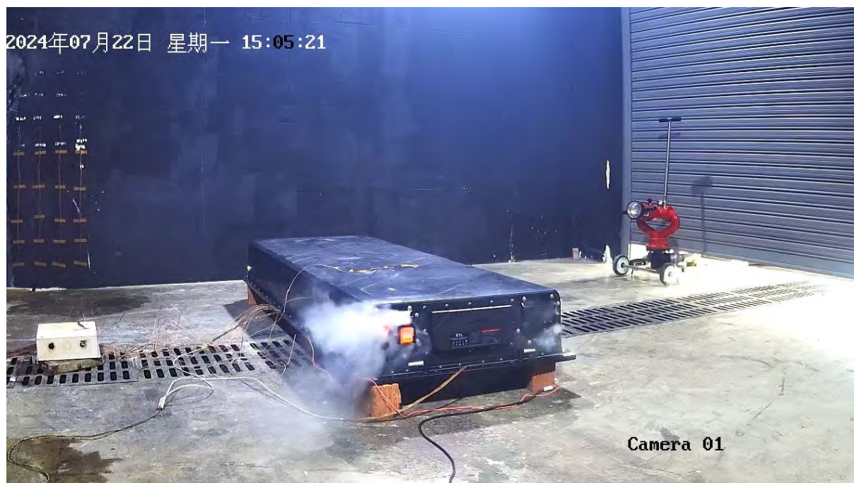
Figure 11. Photo of event (E4) during test.
