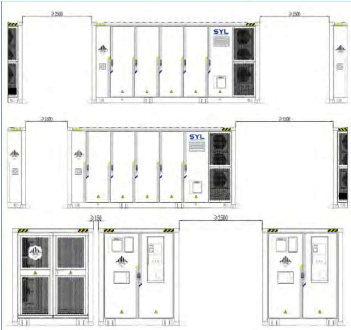
Figure 1.6.1 – ESS Separation Requirements per SYL (Manufacturer)
