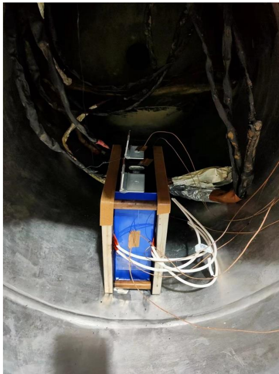
Sample #1: After thermal runaway test
