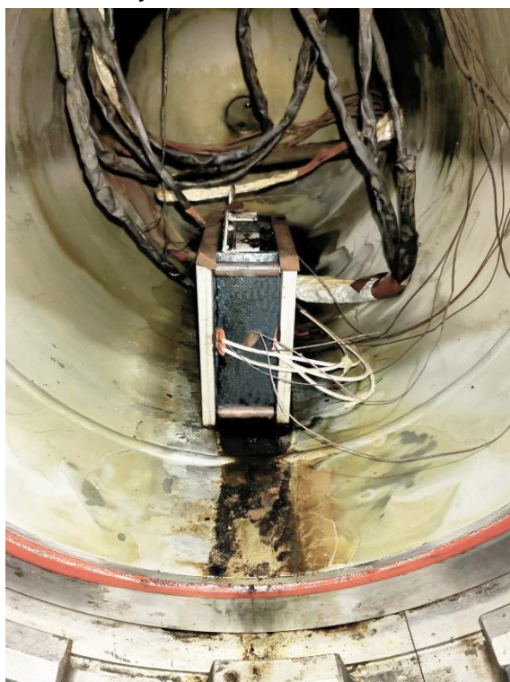
Sample #1: After thermal runaway test
