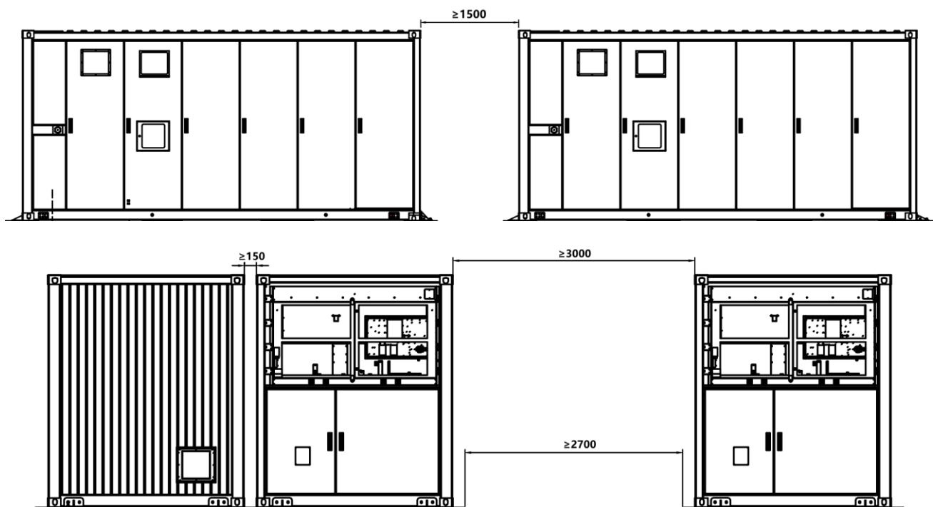
Figure 4-5 Installation Space Requirements for Multiple Container A Units (mm)
