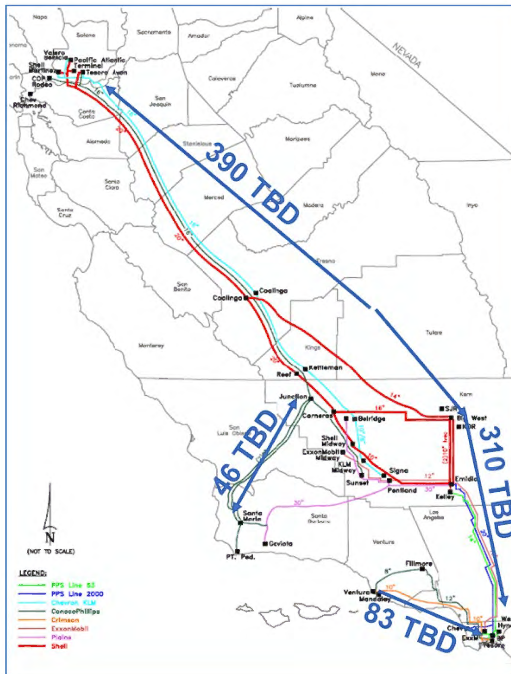
Figure 7 - Location, alignment and carrying capacity of key crude oil pipeline infrastructure
