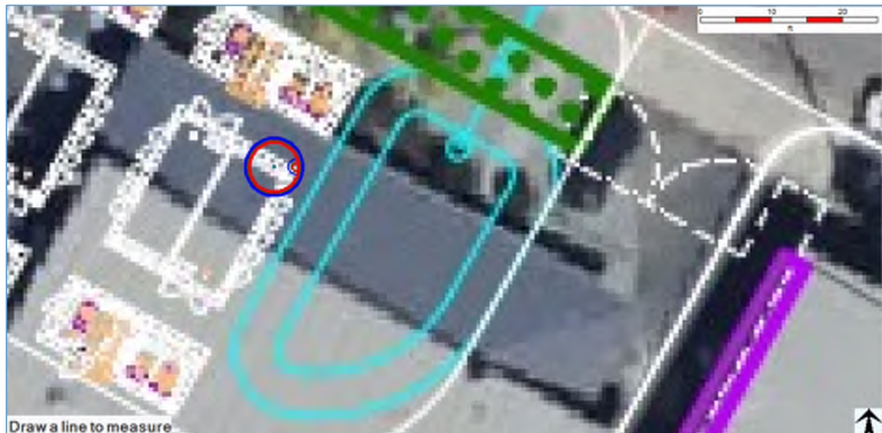
Figure 10.5(b) – UL 9540A Cell-level Test Gas Explosion – Pressure Effects (Large circles show 1.45 psi, 3 psi, and 4.35 psi effect zone contours. Small circles show overpressure event 3-ft offset from gas release point)
