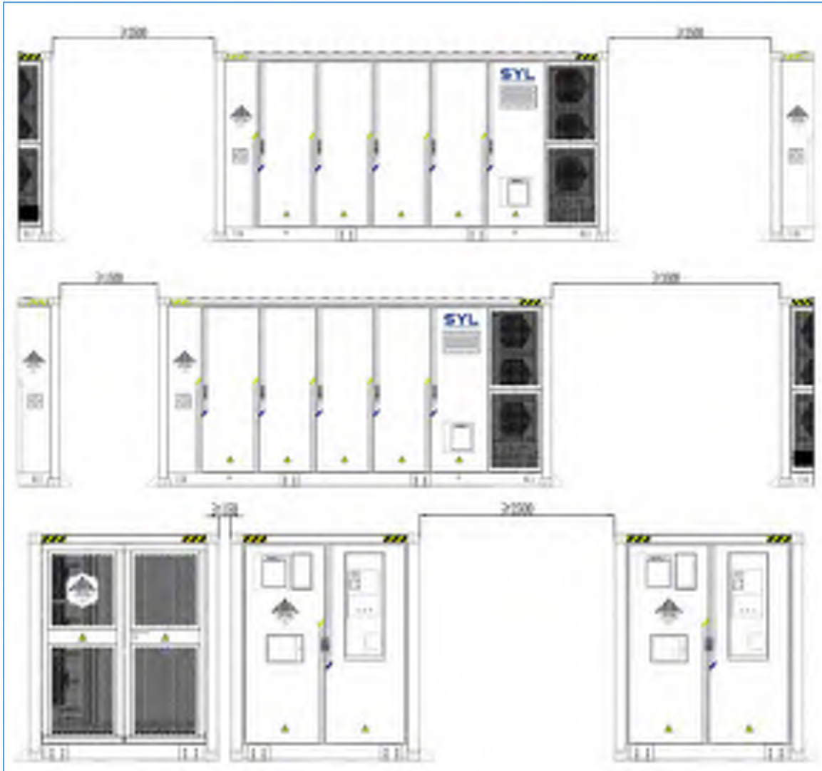
Figure 1.6.1 – ESS Separation Requirements per SYL (Manufacturer)
