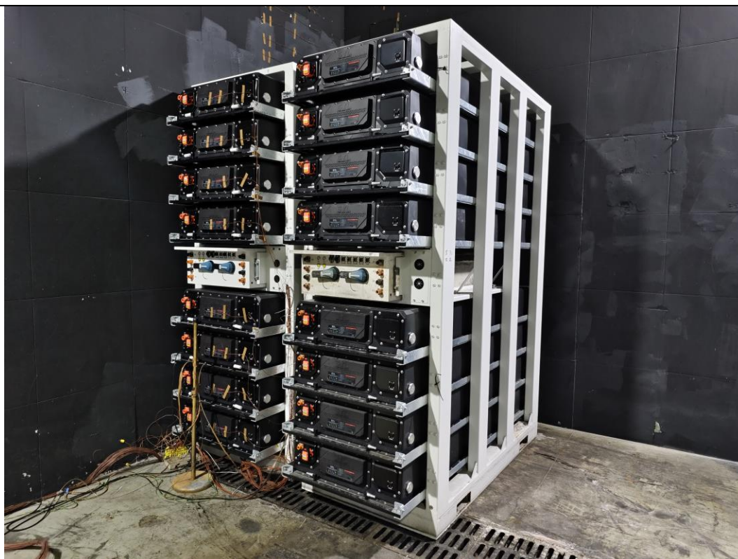
Figure 16. View of positioning of BESS units in testing room.
