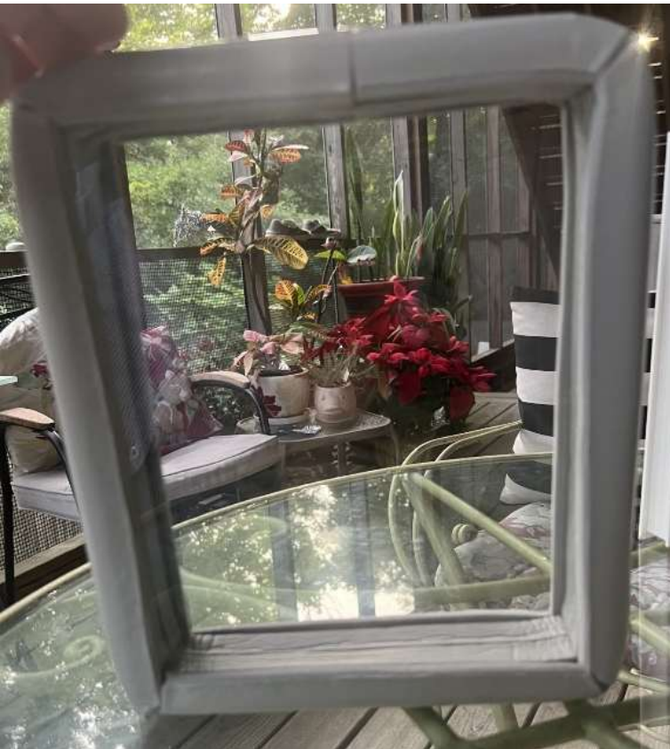
Early stage prototype going into R6.6 fixed window. Latest version has white foam clean edges, caulked at the glazing perimeter to provide a water-&air-tight seal. Low tech delivers AFFORDABLE high performance
