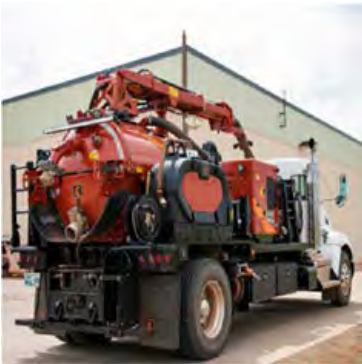
Vacuum Assisted Truck with Pressure Washer
