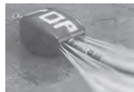
Examples of culvert cleaning nozzles appropriate for Isolator Row PLUS maintenance. (These are not StormTech products).
