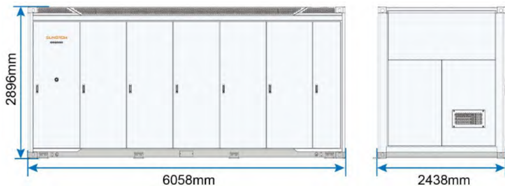
Figure 4-1: Geometry of Sungrow energy storage system
