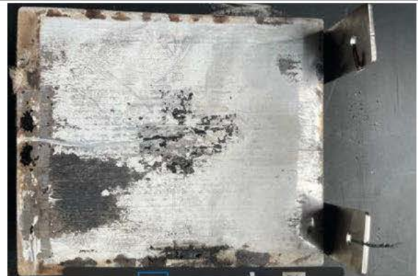
Figure 32: After thermal runaway-1
