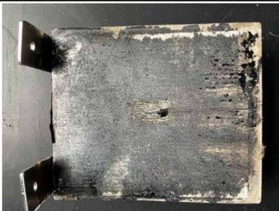
Figure 27: After thermal runaway-2
