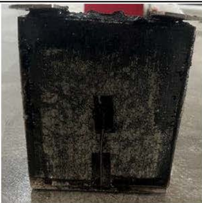
Figure 21: After thermal runaway-2
