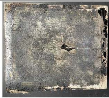
Figure 26: After thermal runaway-1
