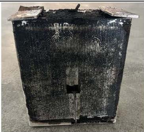
Figure 15: After thermal runaway-2
