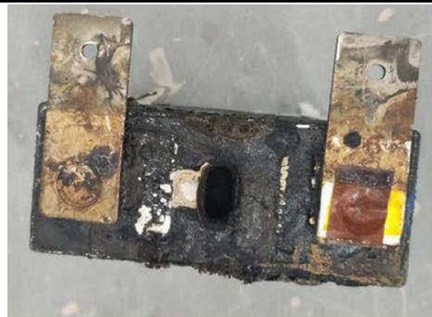
Figure 40: After thermal runaway-4
