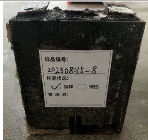
Figure 20: After thermal runaway-1
