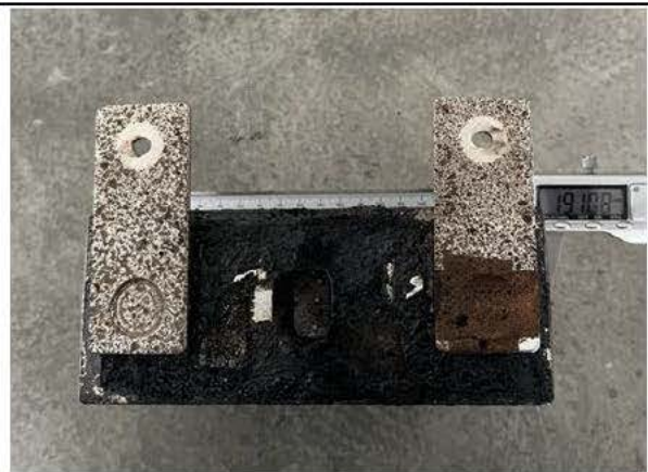
Figure 16: After thermal runaway-3
