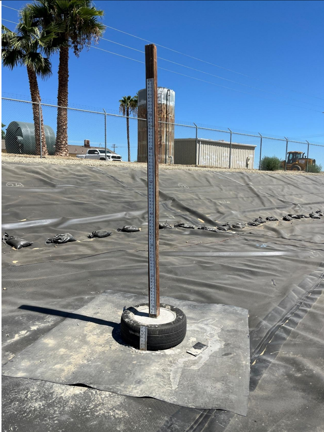
Photograph #13: Water Depth Gauge to 8'.
