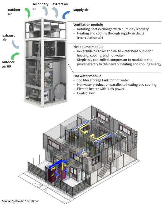
RD&D on mechanical pods for retrofit applications has been carried out previously with CEC funding, for example the "Low-GWP Mechanical Modules for
