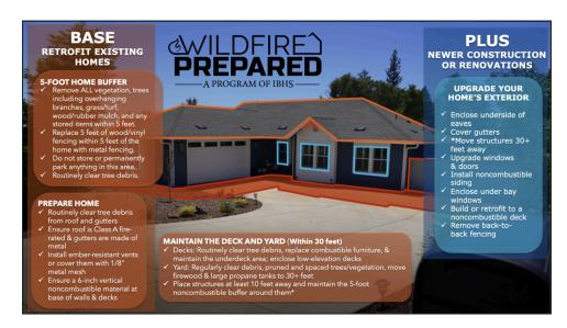
The IBHS Wildfire Prepared standards provide a validated starting point for useful resilience measures that could be systematically incorporated into modular housing.
