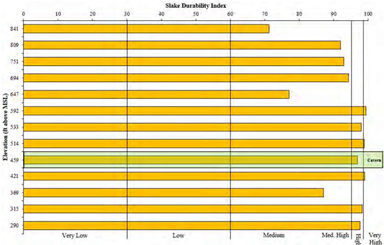
Figure 4-12. Slake Durability Index Recorded in Core Hole ZEV-CH-06-24
