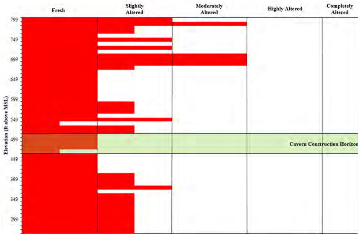
Figure 3-8. Degree of Alteration Logged in Core Hole ZEV-CH-06-24
