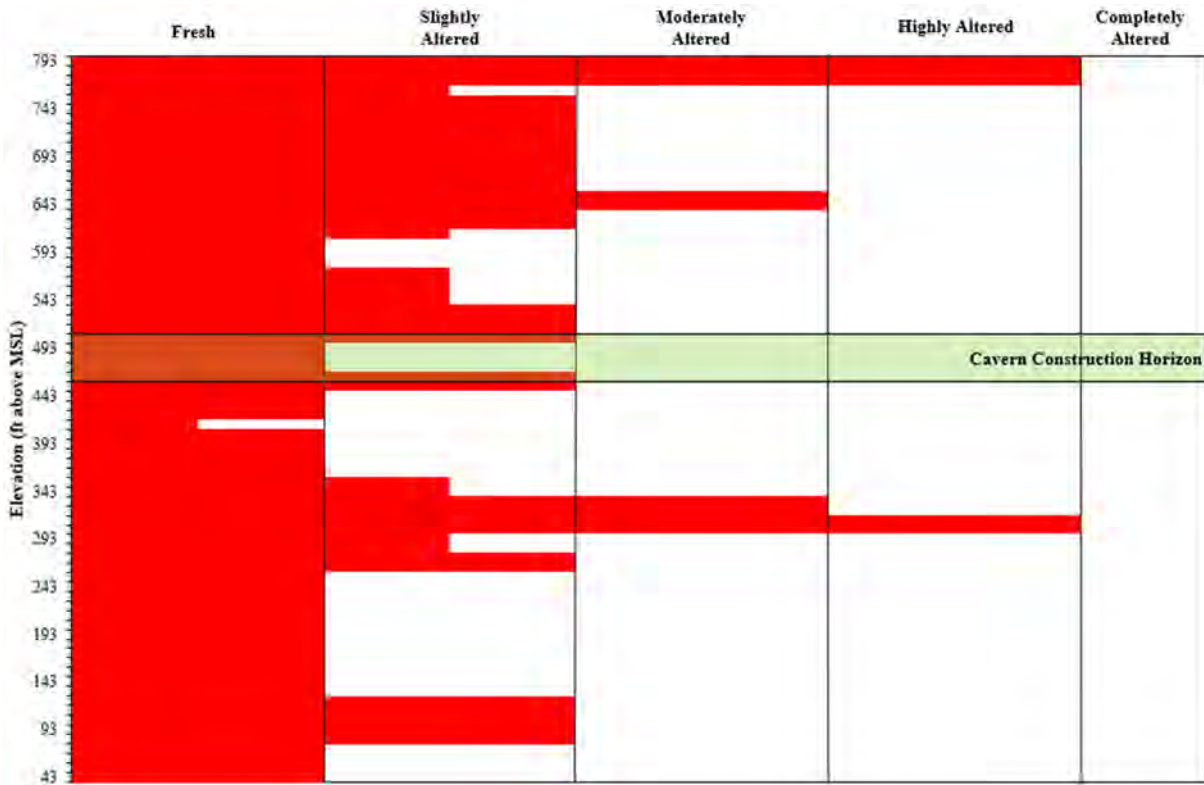
Figure 3-6. Degree of Alteration Logged in Core Hole ZEV-CH-04-24
