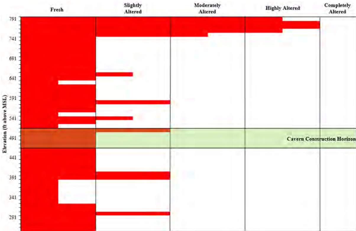
Figure 3-7. Degree of Alteration Logged in Core Hole ZEV-CH-05-24
