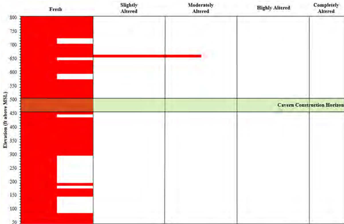
Figure 3-3. Degree of Alteration Logged in Core Hole ZEV-CH-01-23
