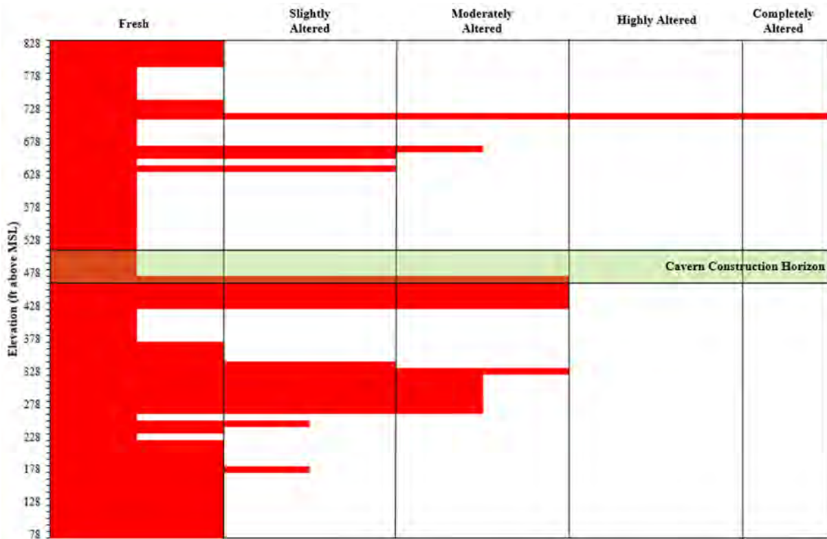
Figure 3-4. Degree of Alteration Logged in Core Hole ZEV-CH-02-23
