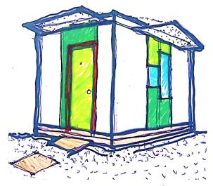
A CBECCS model of a 120sf microhome with 2kw rooftop solar plus a 5kwh battery using the window-integrated envelope has a Time-of-Day Value ("EDR2") 87% lower than the code-compliant Standard Model. This 120sf microhome design has been cost estimated at an AFFORDABLE \$25,000 DIY and \$50,000 contractor built.
