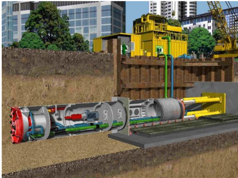
Figure 4 - General layout of pipe jacking with cutting head (courtesy of Cigré TB 770)
