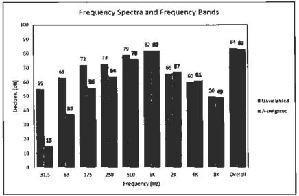
Figure 2: Caltrans Traffic Noise Spectra Showing Differences in Unweighted and Weighted Spectra and Overall Levels<sup>11</sup>
