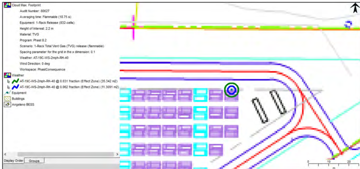
Figure 14. Map of horizontal extent of vapor cloud for LFL (6.2% in blue) and 1/2 LFL (3.1% in green)
