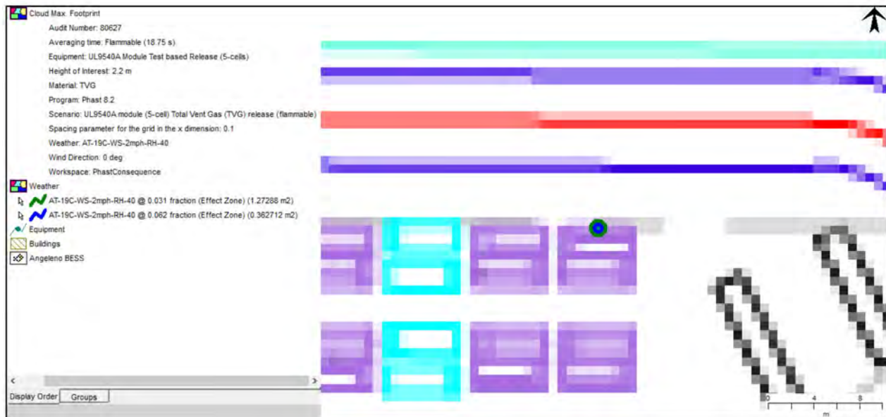
Figure 8. Map of horizontal extent of vapor cloud for LFL (6.2% in blue) and 1/2 LFL (3.1% in green)
