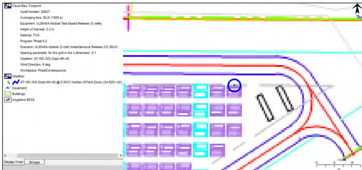
Figure 11. Map of horizontal extent of vapor cloud for CO IDLH (1200 ppm)
