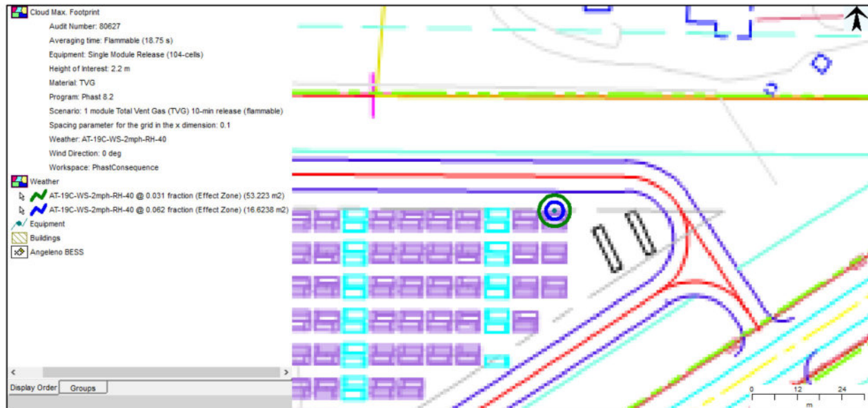
Figure 3. Map of horizontal extent of vapor cloud for LFL (6.2% in blue) and ½LFL (3.1% in green)
