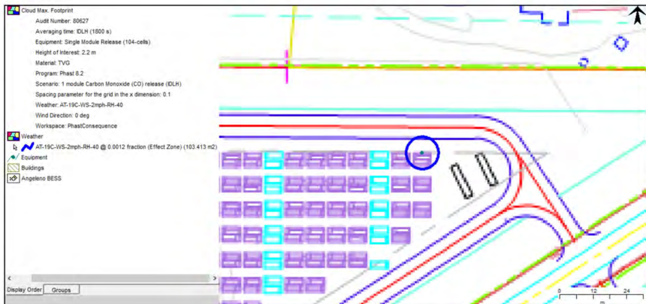
Figure 13. Map of horizontal extent of vapor cloud for CO IDLH (1200 ppm)
