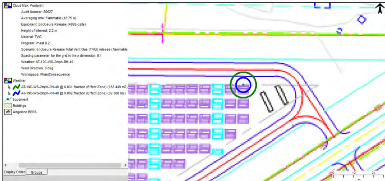
Figure 16. Map of horizontal extent of vapor cloud for LFL (6.2% in blue) and 1/2 LFL (3.1% in green)
