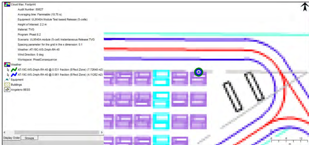
Figure 10. Map of horizontal extent of vapor cloud for LFL (6.2% in blue) and 1/2 LFL (3.1% in green)
