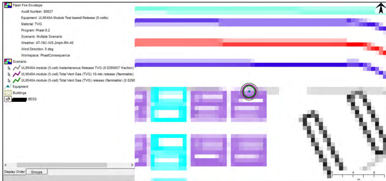
Figure 18. Maximum Extent of Flash Fire Envelope (Duration < 3 sec)
