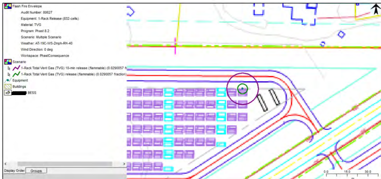
Figure 20. Maximum Extent of Flash Fire Envelope (Duration < 3 sec)
