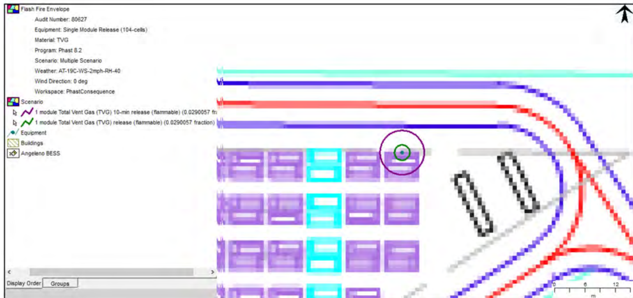
Figure 19. Maximum Extent of Flash Fire Envelope (Duration < 3 sec)
