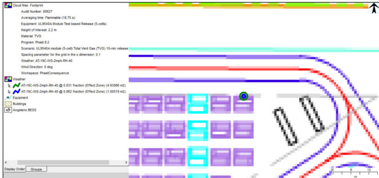
Figure 1. Map of horizontal extent of vapor cloud for LFL (6.2% in blue) and 1/2 LFL (3.1% in green)
