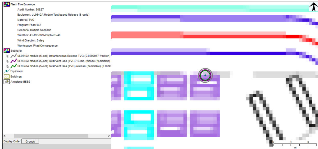
Figure 9. Maximum Extent of Flash Fire Envelope (Duration < 3 sec)
