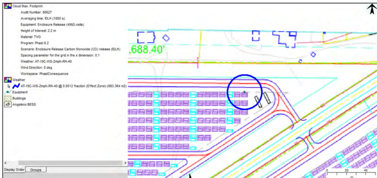
Figure 17. Map of horizontal extent of vapor cloud for CO IDLH (1200 ppm)
