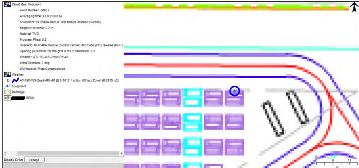
Figure 9. Map of horizontal extent of vapor cloud for CO IDLH (1200 ppm)
