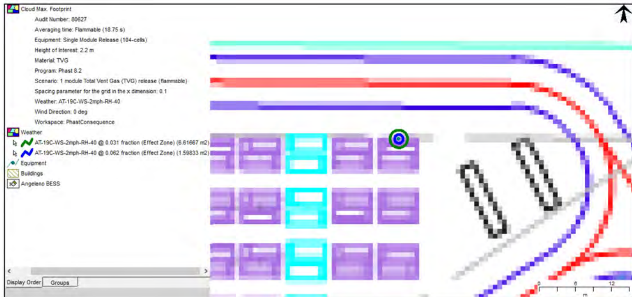
Figure 12. Map of horizontal extent of vapor cloud for LFL (6.2% in blue) and 1/2 LFL (3.1% in green)
